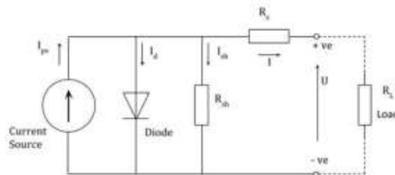
**Fig.2.** Photovoltaic module equivalent circuit
