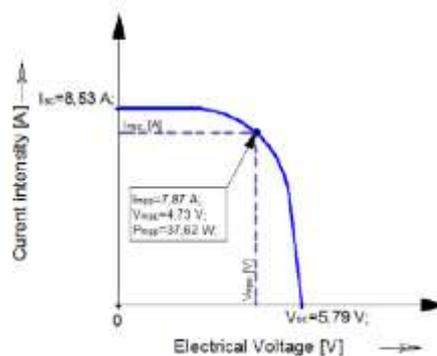
**Fig.4.** Current-Voltage curve of monocrystalline photovoltaic cells used in this study [3]
