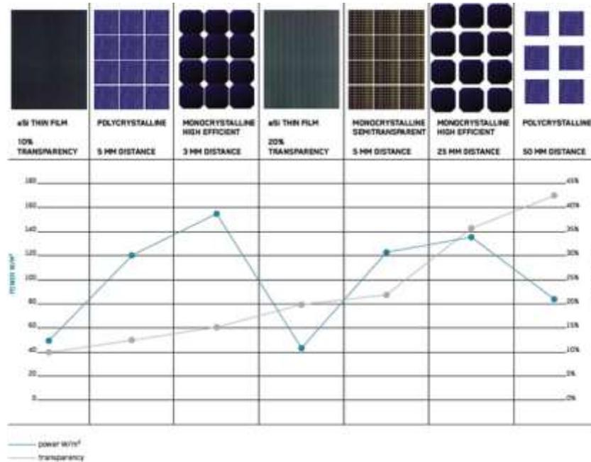
**Fig.3.** Different types of photovoltaic cells used for buildings integrated photovoltaic systems, [7]
