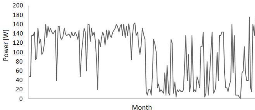
**Fig.6.** Variation of power provided by building integrated photovoltaic system in 2013
