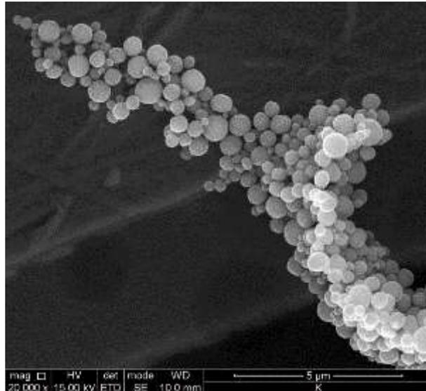
**Fig. 1** SEM image of ZnO particles prepared by the diethylene glycol thermal method.
