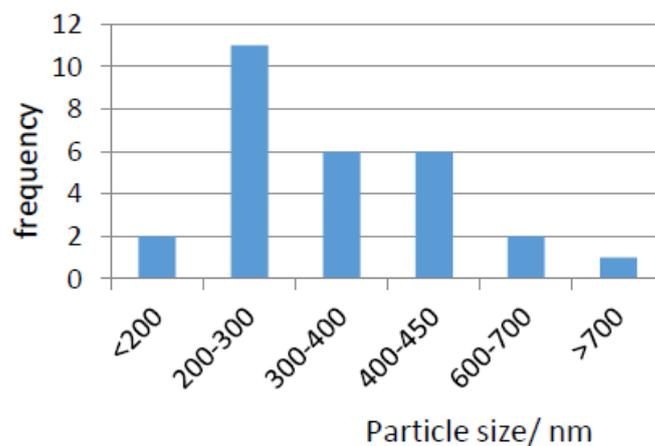
**Fig. 2** Frequency distribution of the size of ZnO particles extracted from the analysis of SEM images.
