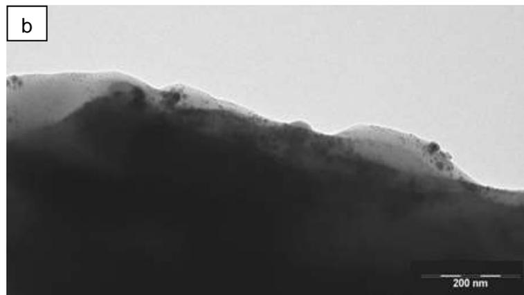
Fig. 7 a) SEM BSE image of PCL/0.5 wt.% HAp fibers b) TEM image of PCL/0.5 wt.% HAp fibers
