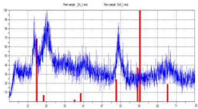
Fig. 2. X-ray diffraction patterns of titanate nanotubes
