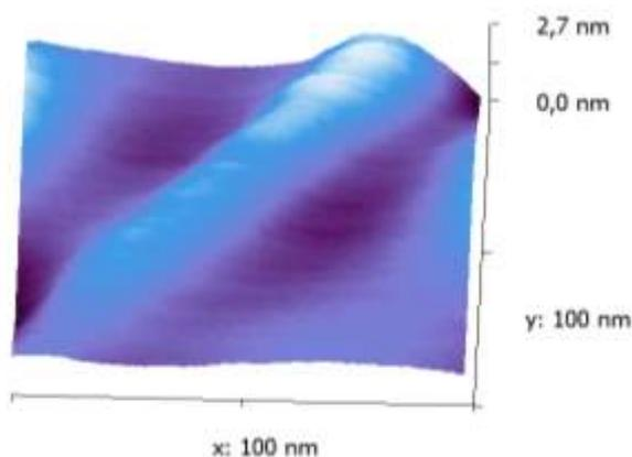
Fig. 9. AFM of pure titanate nanotubes
