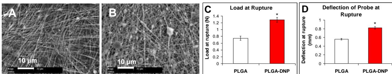
**Fig. 2.** SEM morphology (A, B) and mechanical properties (C, D) of PLGA and PLGA-DNP scaffolds. C, D: Mean  $\pm$  S.E.M. from 10 samples for each experimental group. Two-tailed t-test, \* $p \leq 0.05$  compared to PLGA.
