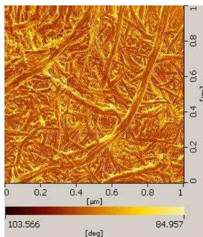
Figure 1 AFM image of dried suspension of CNF.
