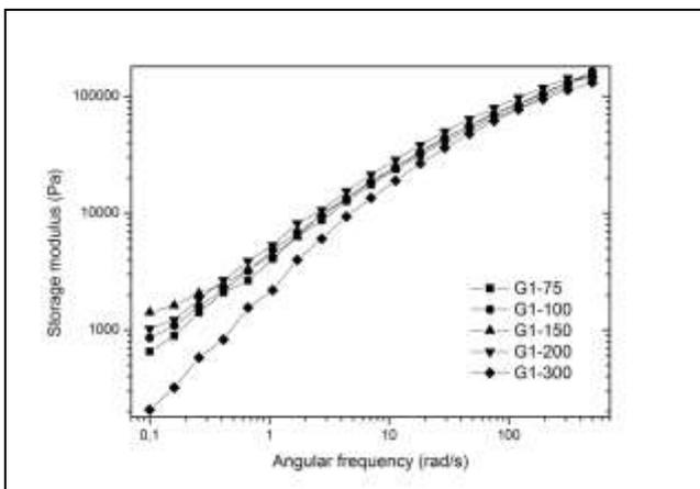
**Fig. 5: Melt elasticity of nanocomposites (G2)**
