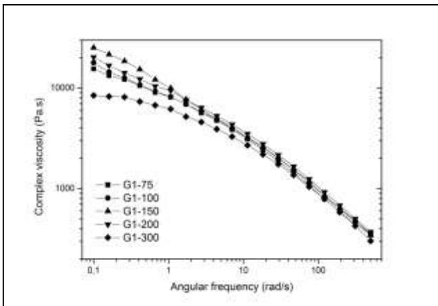
**Fig. 2: Viscosity curves of nanocomposites (G1)**
