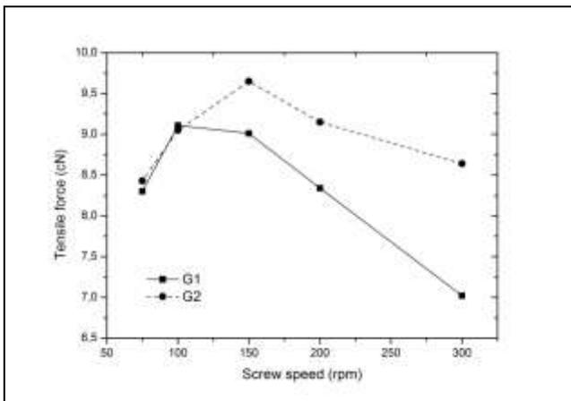
**Fig. 1: Melt strength level of nanocomposites**
