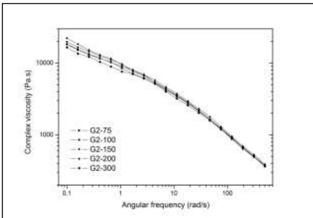
**Fig. 4: Viscosity curves of nanocomposites (G2)**
