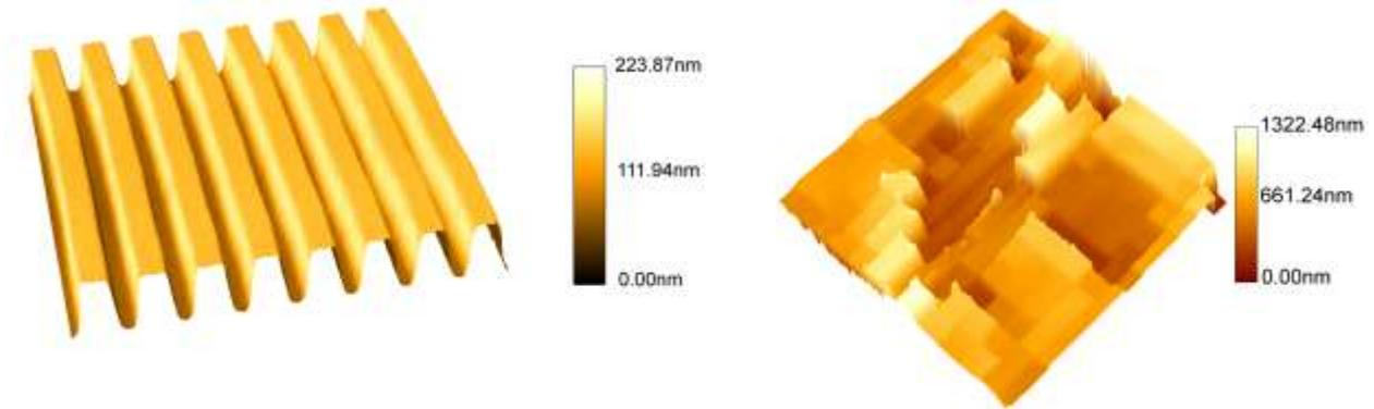
**Fig. 3** Binary period gratings (ratio 1:1 between exposed and unexposed areas) with period 1  $\mu\text{m}$  (left), and multileveled structures (computer generated holograms) 25  $\mu\text{m}$   $\times$  25  $\mu\text{m}$  (right).
