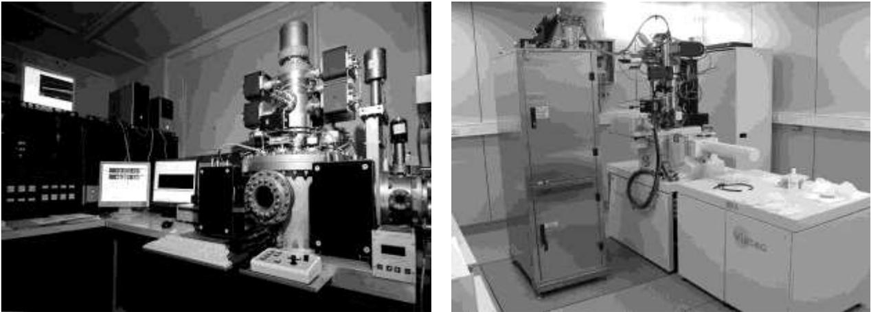
**Fig. 1** Variable shaped e-beam lithography system BS600 (left) and Gaussian e-beam lithography system Vistec (right).
