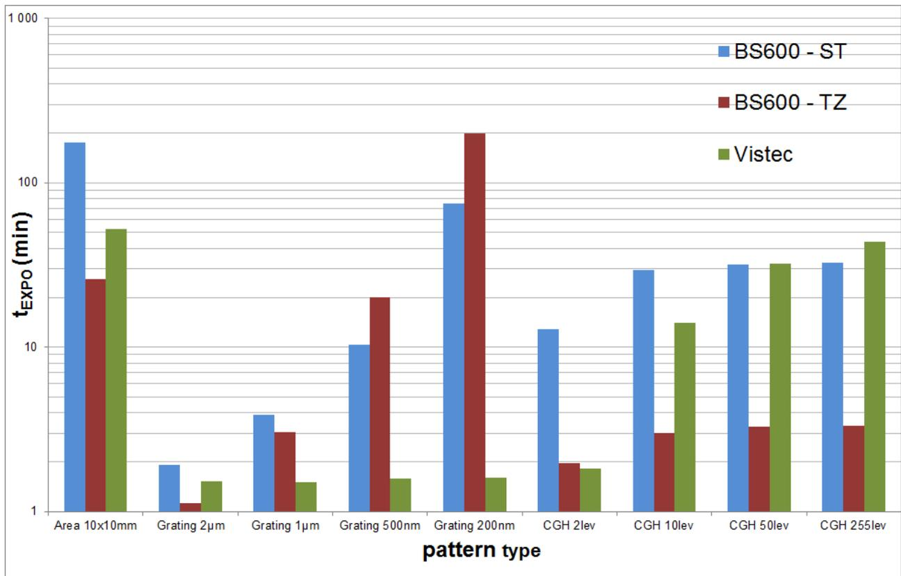
**Fig. 4** Exposure time comparison for variable shaped beam lithography system BS600 and Gaussian beam lithography system Vistec on various pattern types (continuous area of 10 mm  $\times$  10 mm, gratings with periods 2  $\mu\text{m}$ , 1  $\mu\text{m}$ , 500 nm, 200 nm and multilevel structures with 2, 10, 50 and 255 levels).
