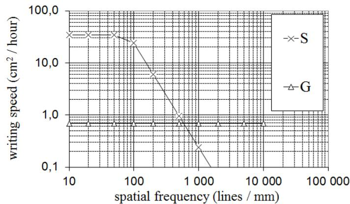
**Fig.2** Writing speed comparison between shaped beam lithography system (S) and Gaussian beam lithography system (G).
