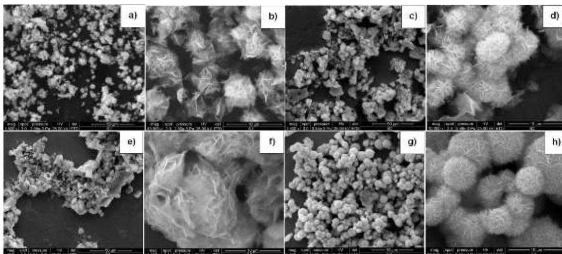
**Fig. 2** SEM images of S1 (a, b), S2 (c, d), S3 (e, f) and S4 (g, h) at 1,500 and 10,000 X.
