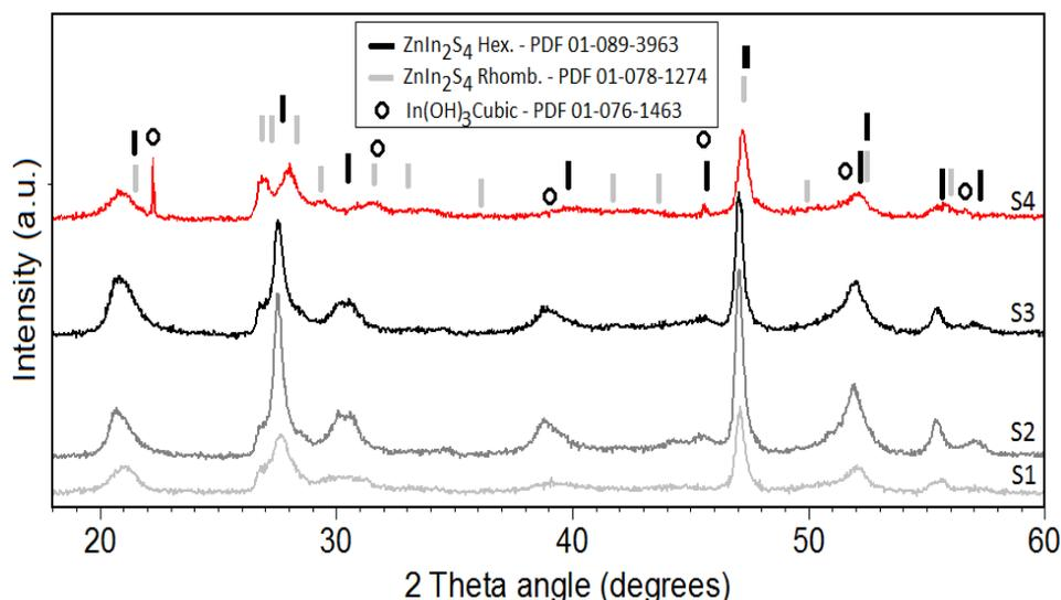
Fig. 1 XRD pattern of  $\text{ZnIn}_2\text{S}_4$  samples.
