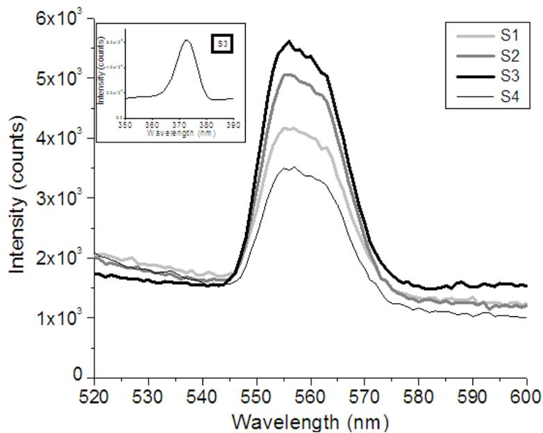
**Fig. 5** Photoluminescence spectra of  $\text{ZnIn}_2\text{S}_4$  samples and excitation spectra - inset.
