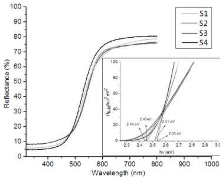
**Fig. 4** UV–vis diffuse reflectance spectra of ZnIn<sub>2</sub>S<sub>4</sub> samples.
