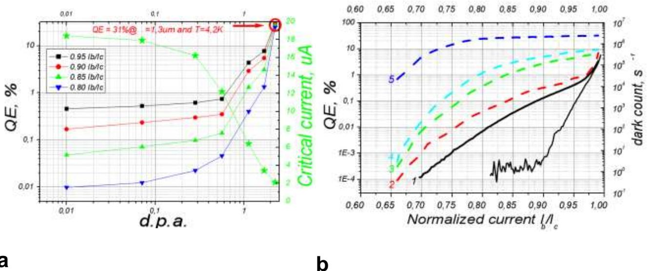
**Fig. 2. a)** Dependence of QE and critical current versus displacement per atom (d.p.a.). **b)** Dependence of QE and dark count rate versus normalized current. The curves 1 (solid black), 2 (dash red), 3 (dash green), 4 (dash cyan), 5 (dash blue) correspond to doses 0, 0.6, 1.14, 1.7, 2.25 d.p.a., respectively
