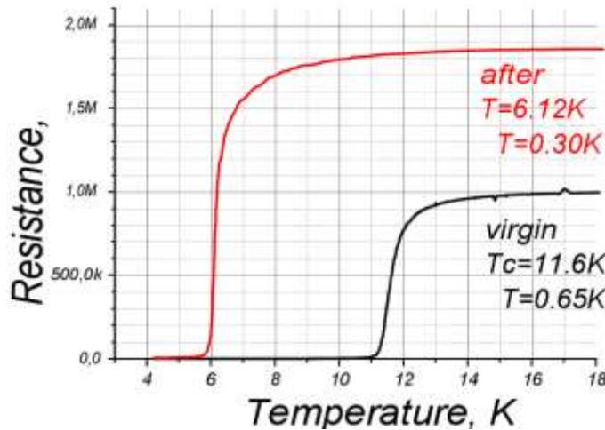
**Fig. 1.** Dependence of SSPD resistance versus temperature before and after proton irradiation (at optimal dose). The black curve – virgin (before irradiation) and the red curve – after irradiation (d.p.a. is 2.1)
