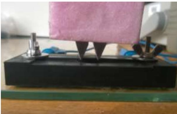
**Fig. 2** Dielectric electrodes
