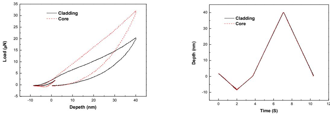
**Fig. 1** Experimental design of POF core and cladding under 40 nm maximum depth, 400 nm spacing, 10 s loading time and 10 s holding time: typical load-depth curve (left) and depth-time curve (right).
