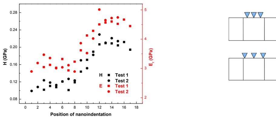
**Fig. 6** Hardness and elastic modulus with 40 nm depth and 400 nm spacing (left); Possibilities of three indents in the interphase region (right)
