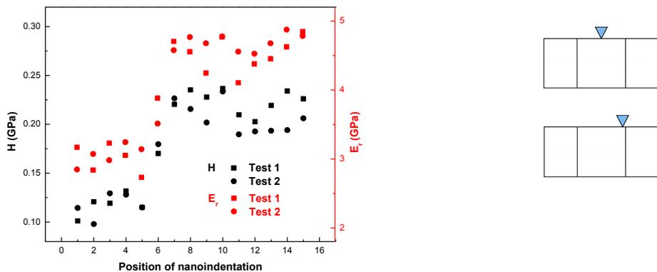
**Fig. 4** Hardness and elastic modulus with 80 nm depth and 1300 nm spacing (left); Possibilities of one indent in the interphase region (right)
