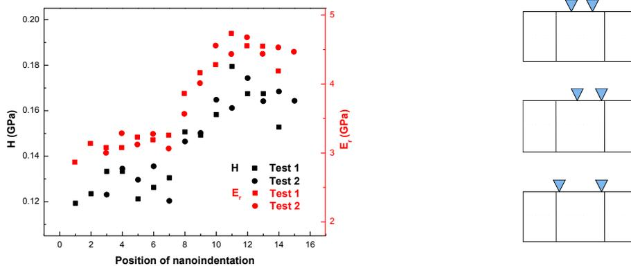
**Fig. 5** Hardness and elastic modulus with 40 nm depth and 700 nm spacing (left); Possibilities of two indents in the interphase region (right)
