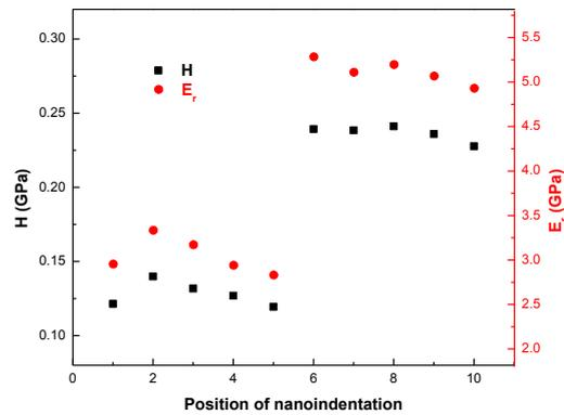
**Fig. 3** Hardness and elastic modulus with 120 nm depth and 1900 nm spacing
