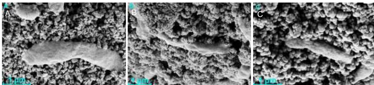
**Fig. 4** Scanning electron microscope images showing (A) *Escherichia coli* colonizing the surface of aggregated diamond nanoparticles; (B) *E. coli* colonizing SiO<sub>2</sub> nanoparticles, and (C) *E. coli* colonizing TiO<sub>2</sub> nanoparticles.
