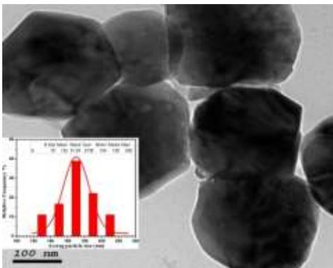
**Fig. 9(a) TEM image of annealed sample at  $T_a = 700^\circ\text{C}$  and the corresponding histogram on the inset**
