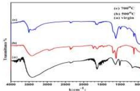
**Fig. 2 FTIR spectra for as prepared ZnS and annealed samples at  $T_a = 500$  °C and  $700$  °C**
