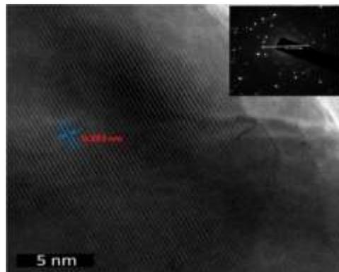
**Fig.9 (b) HRTEM image and SAED for annealed ZnS nanoparticles at  $T_a = 700^\circ\text{C}$**
