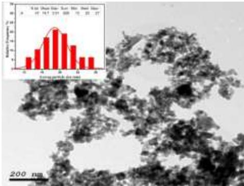
**Fig. 8 (a) TEM image and the corresponding histogram of annealed ZnS at  $T_a = 500^\circ\text{C}$**
