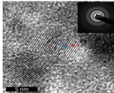
**Fig. 7(b) HRTEM image and SAED for as prepared ZnS nanocrystallites**
