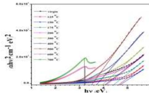
**Fig. 3(b) plots of  $(\alpha hv)^2$  versus  $hv$  at different  $T_a$ , the inset represents dependence of  $E_g^{opt}$  and  $D$  on  $T_a$**
