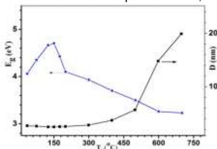
**Fig. 3(c) Dependence of  $E_g^{opt}$  and  $D$  on annealing temperatures**
