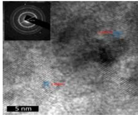
**Fig. 8(b) HRTEM image and SAED for annealed ZnS at  $T_a = 500^\circ\text{C}$**
