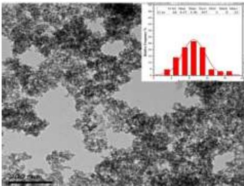
**Fig. 7(a) TEM image of as prepared ZnS nanoparticles and histogram on the inset**
