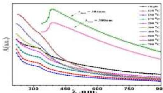
**Fig. 3(a) Optical absorption spectra for as prepared and annealed samples of ZnS nanoparticles at different  $T_a$**
