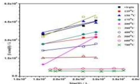
Fig. 1(b) Plot of  $\beta \cos \theta / \lambda$  vs.  $\sin \theta / \lambda$  of ZnS nanoparticles at different annealing temperatures.
