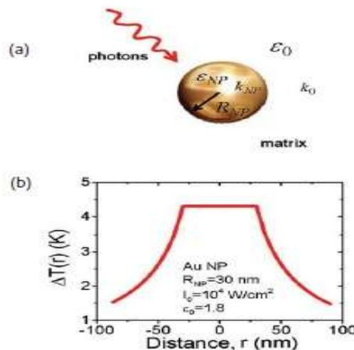
**Fig. (1)** (a) Schematic of an optically driven spherical NP, (b) Calculated temperature increase for a single Au NP as a function of the distance from the NP center. The surrounding medium is water.
