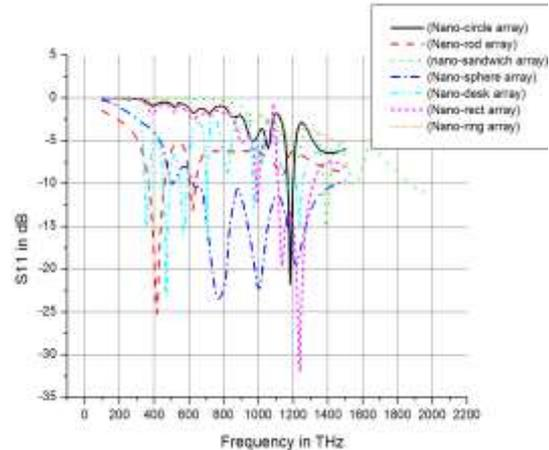
Fig. (3): The  $S_{11}$  versus frequency for all array elements shapes
