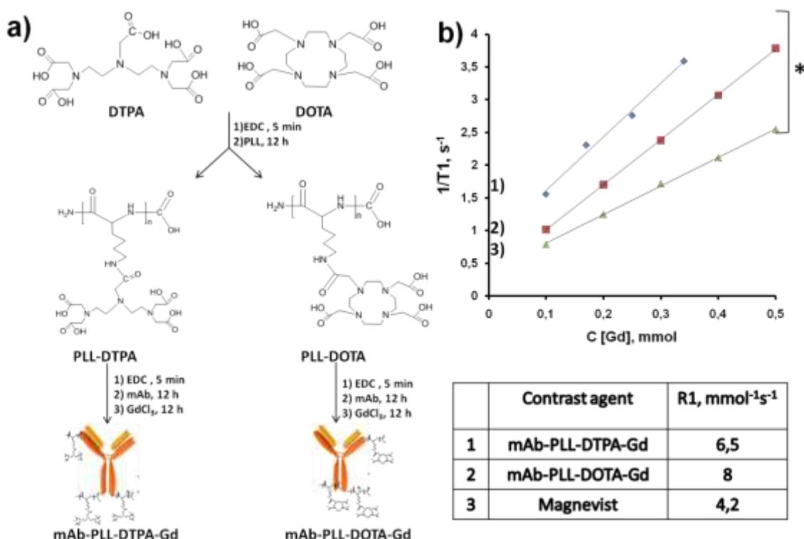
**Fig. 1.** Scheme of synthesis (a) and relaxivity measurements (b) of obtained contrast agents: 1) mAb-PLL-DOTA-Gd; 2) mAb-PLL-DTPA-Gd and 3) Magnevist.
