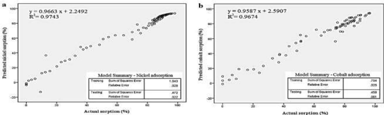
**Fig. 4.** Comparison of model results and the actual removal efficiency (b and c).
