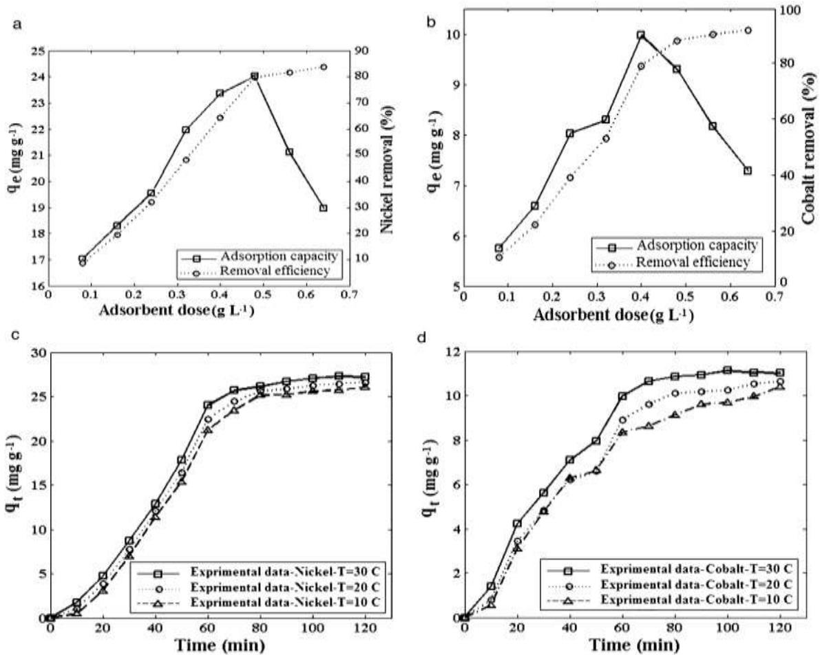
**Fig. 3.** Effect of adsorbent dose on the removal efficiency (% removal) and the adsorption capacity of chitosan/PVA nanofiber membranes for nickel (a) and cobalt (b). Effect of contact time on adsorption capacity of chitosan/PVA nanofiber membranes for nickel (c) and cobalt (d) at different temperatures: 30°C, 20°C and 10°C.
