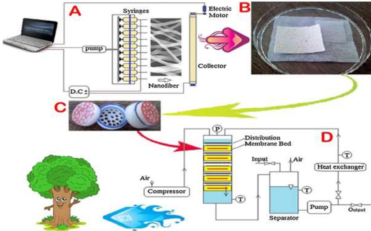
**Fig. 1.** Schematic of the electrospinning process (a), non-woven polyester web before electrospinning process and, chitosan/PVA nanofiber membrane produced on the non-woven polyester web after electrospinning process (b), membrane module (c), schematic of adsorption process.
