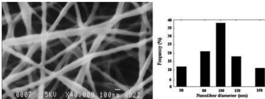
**Fig. 2.** The SEM image and diameter distribution of chitosan/PVA nanofiber membranes.
