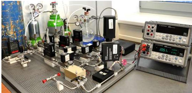
Fig. 5 Gas flow station for sensors characterization
