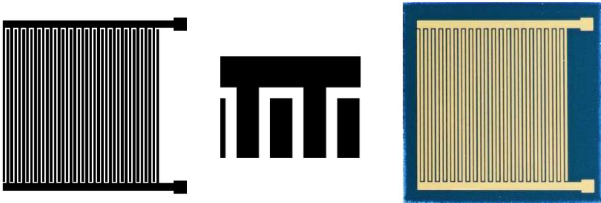
**Fig. 3** Interdigitated structure: design (left), its detail (middle) and fabricated sample (right)
