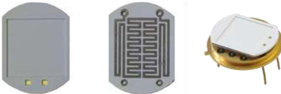
**Fig. 1** LTCC frame (left) / heater (middle) and its placement in the TO-8 package (right)
