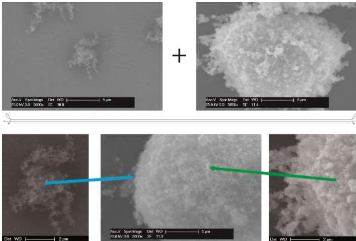
Fig.4 – Particles R972 (top left and bottom) and TiO<sub>2</sub> (top right and bottom) and modified particle TiO<sub>2</sub> particle R972 (bottom middle).
