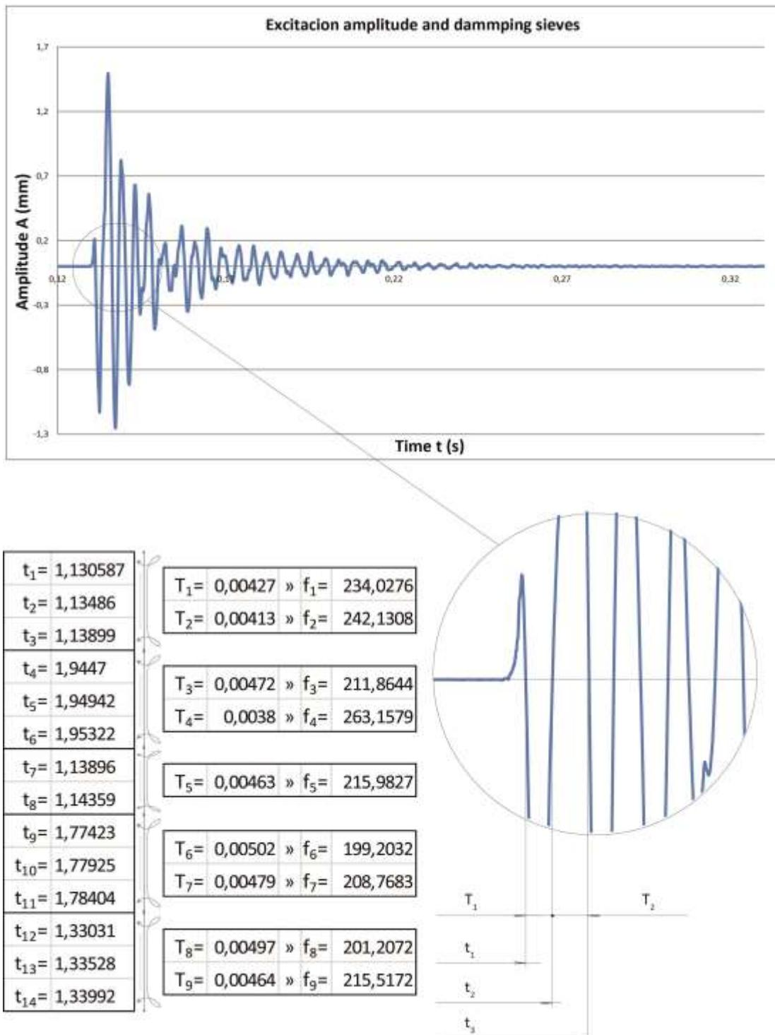
Fig.3 – Example measurements of excited sieve.
