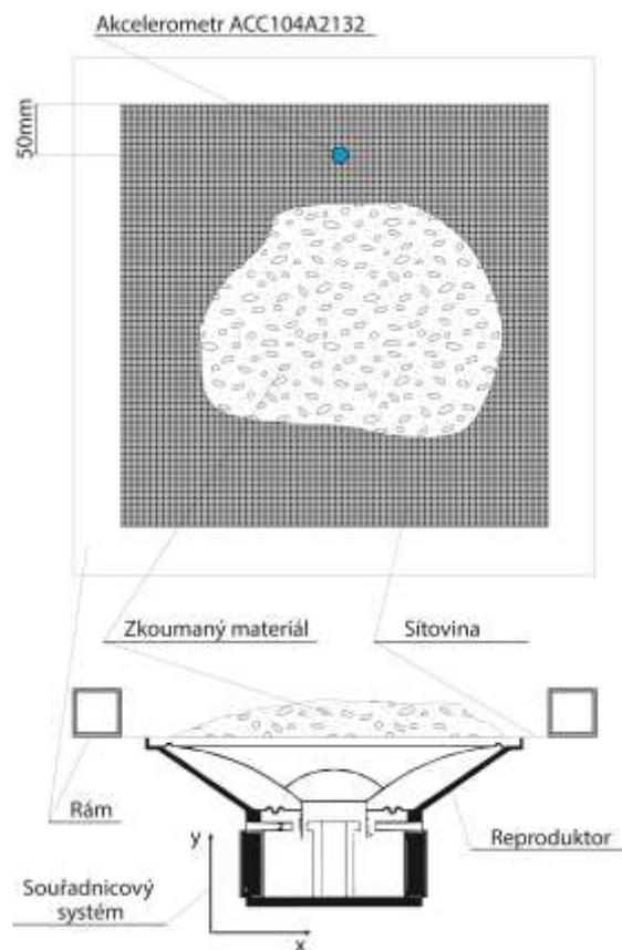
Fig. 2 – Scheme of the experimental equipment.
