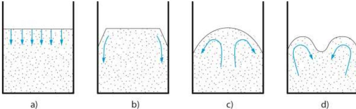
Fig. 1 – Flow pattern of vibrating powder bed.
