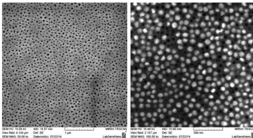
**Figure 2 SEM images of alumina template (magnification 50 kx, left) and deposited gold into the nanoporous template (magnification 100 kx, right)**
