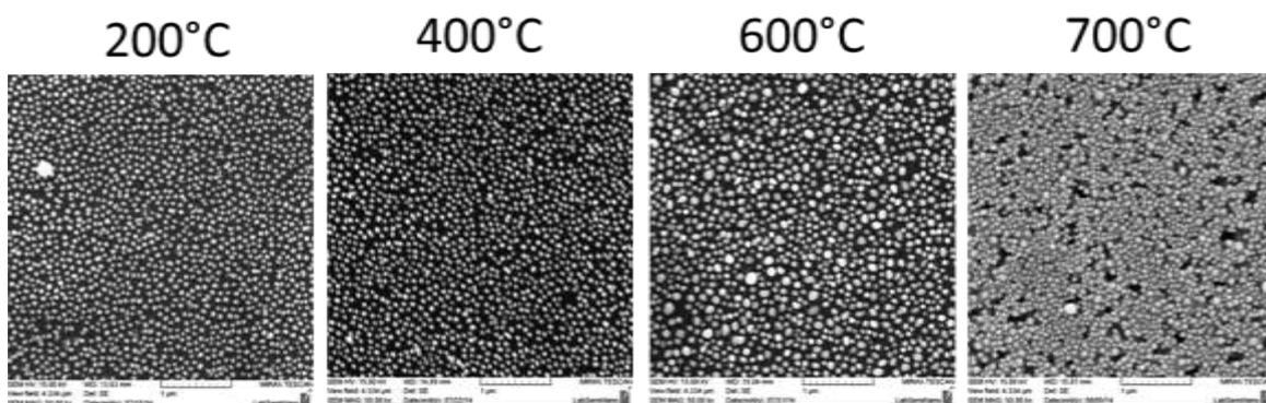
**Figure 4 SEM microimages of atmospheric pressure annealing at various temperatures**
