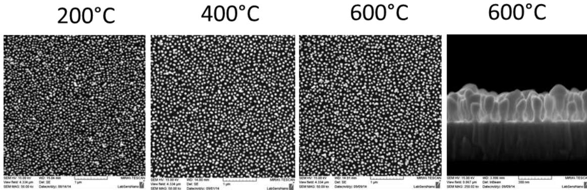
**Figure 5 SEM microimages of vacuum annealing at various temperatures and cross section image for structures after vacuum annealing at 600°C**
