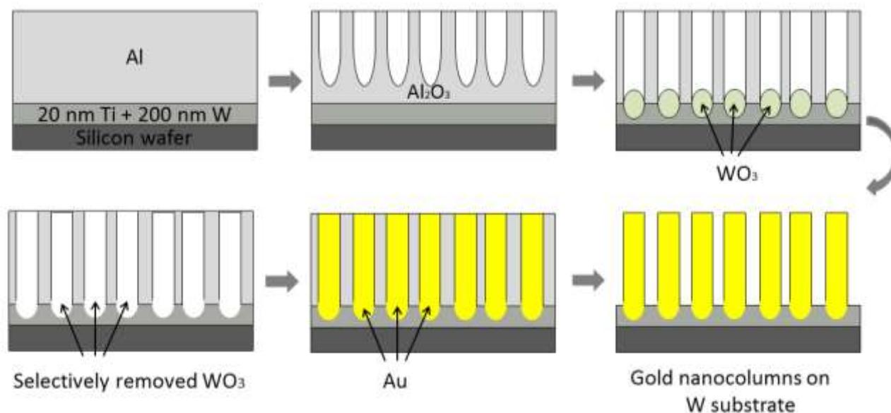
**Figure 1** Scheme of production of gold nanostructured surfaces
