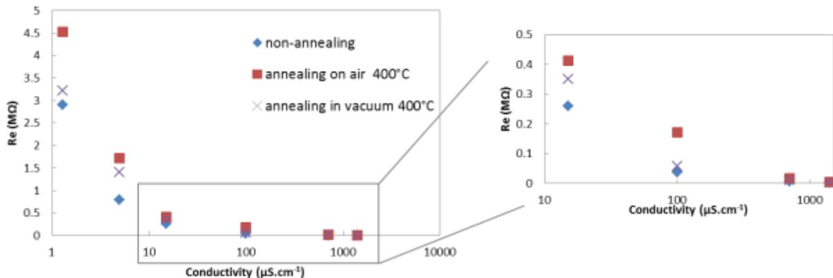
**Figure 7 Dependencies of impedance minima on the concentration of solution for all types of treated surfaces**
