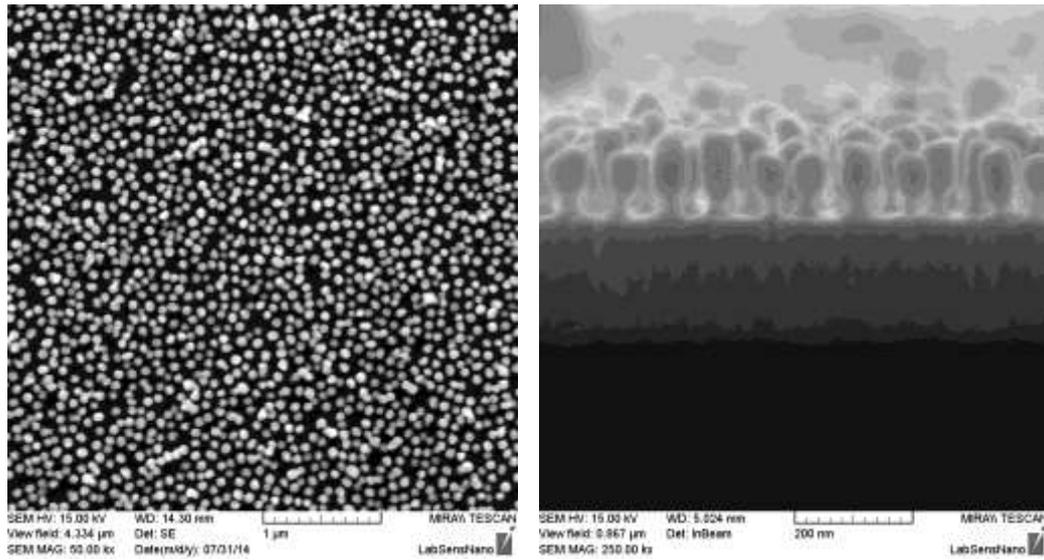
**Figure 3 Gold nanostructures from top view (magnification 50 kx, left) and cross section of gold nanostructured surface (magnification 250 kx, right)**
