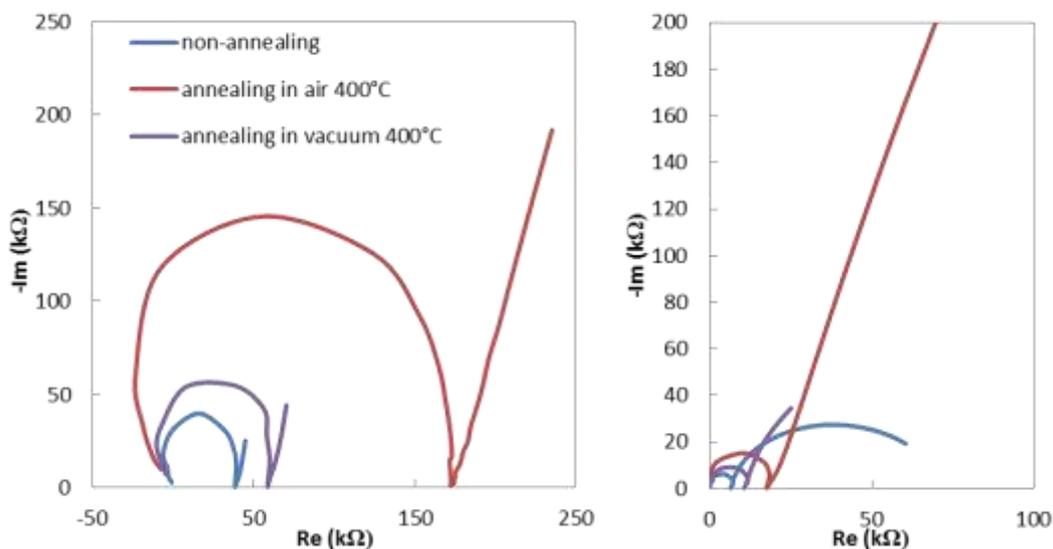
**Figure 6 Impedance spectra for all types of treated surfaces measured in two concentrations of conductivity solutions:  $100 \mu\text{S}\cdot\text{cm}^{-1}$  (left) and  $706 \mu\text{S}\cdot\text{cm}^{-1}$  (right)**
