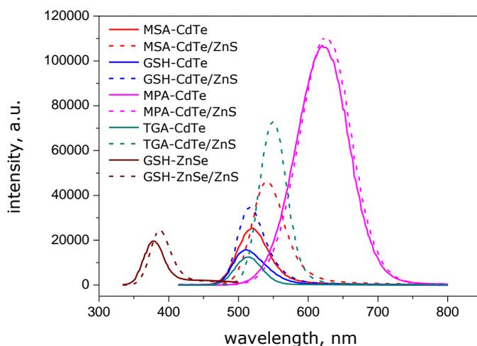
**Fig. 1** Fluorescence spectra of prepared different types QDs
