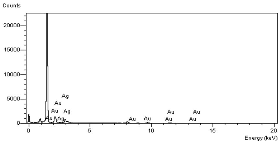
**Figure 2:** SEM image and EDX spectrum of Au coated Ag nanowire by using  $[\text{Au}(\text{en})_2]\text{Cl}_3$  complex
