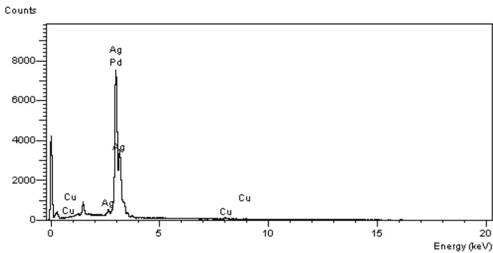
**Figure 1:** SEM image and EDX spectrum of Pd coated Ag nanowire by using  $[Pd(en)_2]Cl_2$  complex
