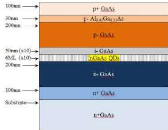
**Fig. 1** Schematic diagram of InGaAs/GaAs quantum dots sample structure.
