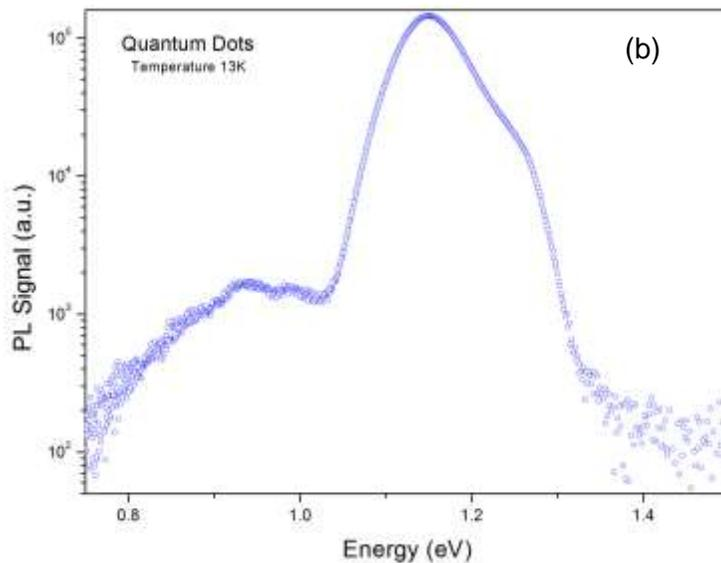
Fig. 2 (a) PL spectra of InGaAs/GaAs quantum dots at different temperatures and (b) shows single spectrum taken on temperature at 13K for analysis.
