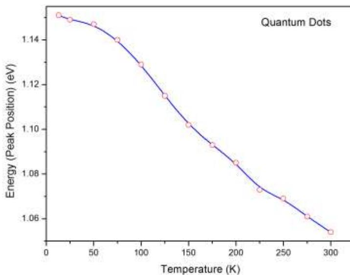
Fig. 3 Temperature dependent peak position of luminescence from InGaAs/GaAs quantum dots.
