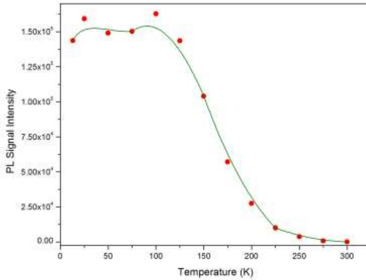
Fig. 4 Temperature dependent PL peak intensity from InGaAs/GaAs quantum dots.
