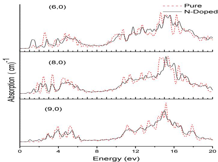
**Fig. 3:** Absorption spectra of (6,0) ; (8,0) and (9,0) pure and doped.
