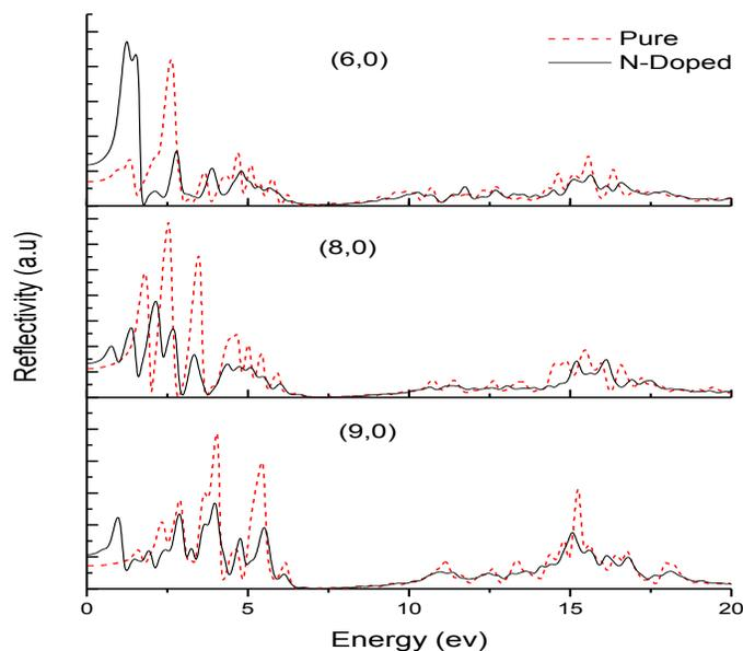
**Fig. 2:** Reflection spectra of (6, 0); (8, 0) and (9, 0) pure and doped SWNT
