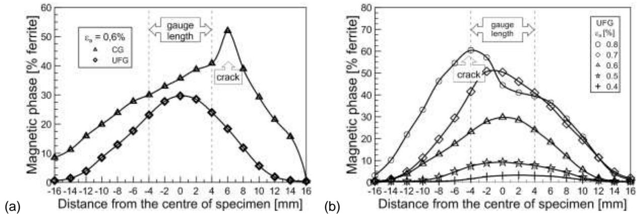
**Fig. 4:** A profile of magnetic phase content along the specimen length. (a) Comparison of CG and UFG materials cycled with the same strain amplitude. (b) Magnetic phase in UFG material cycled with various strain amplitudes.
