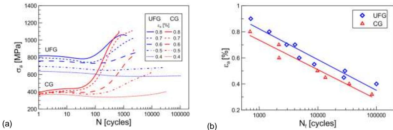
**Fig. 2:** (a) Plot of the stress amplitude  $\sigma_a$  vs. number of cycles  $N$  of AISI 301LN cycled with different  $\epsilon_a$  for CG and UFG materials. (b) Fatigue life curves for UFG and CG materials.
