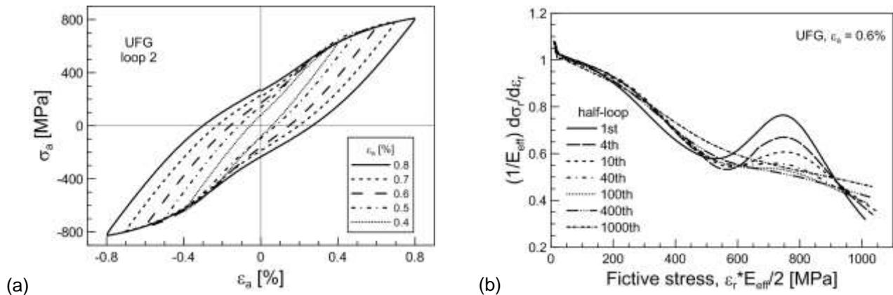
**Fig. 3:** (a) Hysteresis loops of the first closed hysteresis loop at various levels of applied strain amplitude for UFG material. (b) Plot of the first derivative showing the disappearance of the constriction of the loop with increasing number of cycles.
