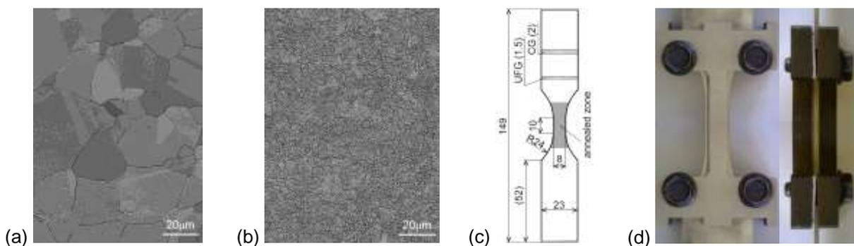
**Fig. 1:** (a, b) Microstructure of CG and UFG material after TMT showing fully austenitic microstructure, equiaxed grains and typical annealing twins in case of CG material, (c) shape of the flat dog-bone specimen with dimensions in mm, (d) special anti-buckling fixtures.
