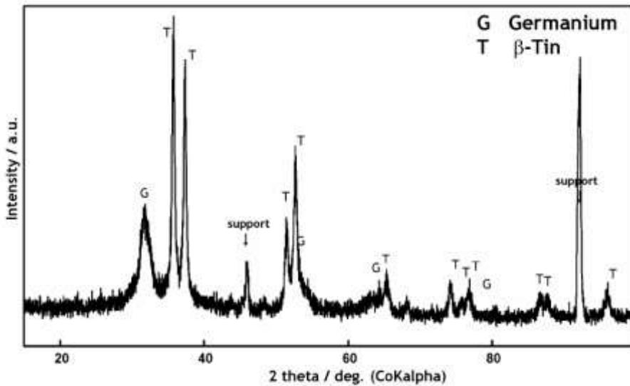
**Fig. 3**  $\mu$ -XRD analysis of the deposit.
