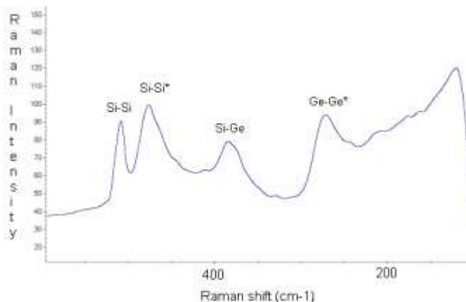
**Fig. 2** Typical Raman spectrum of the Si-Ge-Sn deposit showing Si-Si, Si-Si\*, Si-Ge and Ge-Ge\* peaks.
