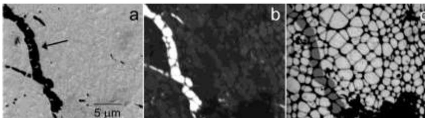
**Fig. 8** Empty hole in the graphene (see arrow) shown at 70 eV in backscattered electrons (a) and at 70 eV (b) and 600 eV (c) in transmitted electrons.
