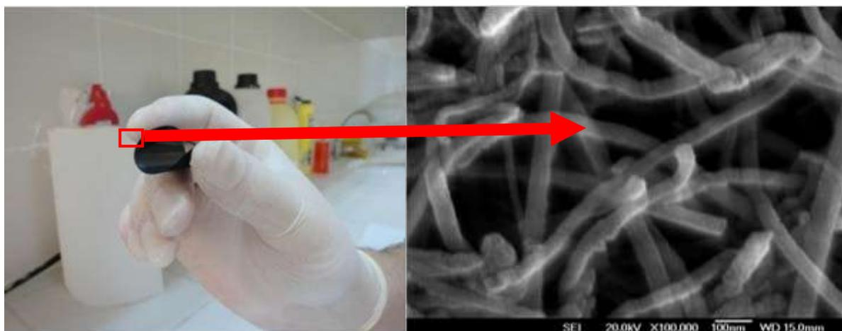
Figure 1. a) Flexible free-standing MWCNT buckypaper and b) FESEM image of buckypaper.
