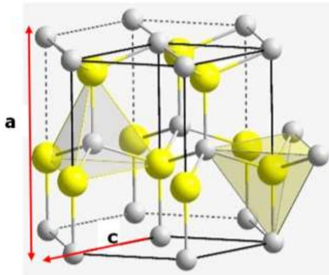
Figure 5. The hexagonal wurtzite ZnO crystal structure.
