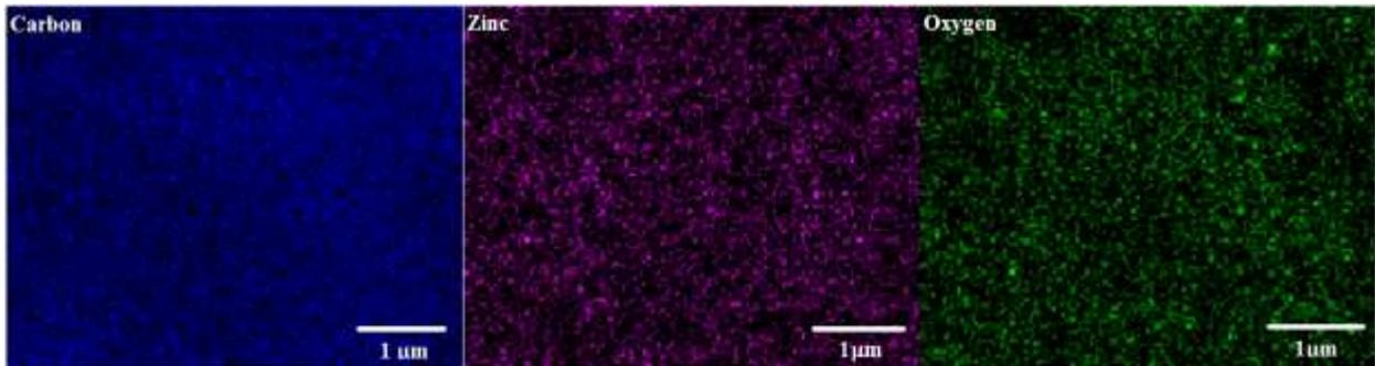
Figure 3. Surface EDS dot-mapping of ZnO/MWCNT nanocomposite electrode.
