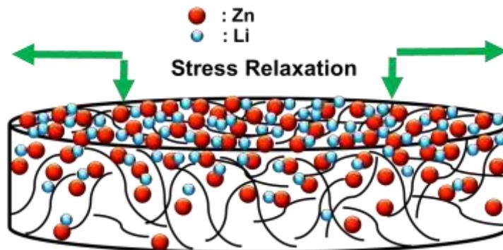
Fig. 10. Stress relaxation mechanism in the nanocomposite electrodes due to MWCNT reinforcement and FGM structure
