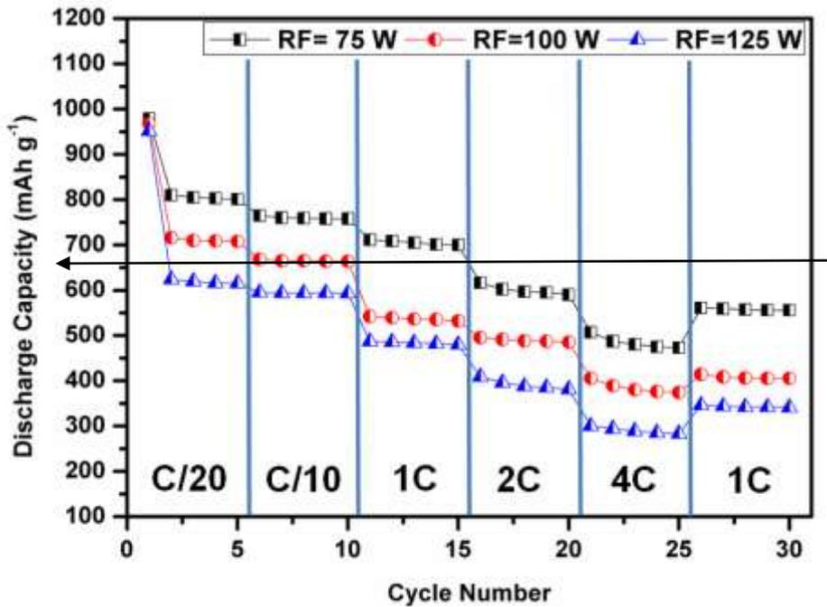
Fig. 9. Rate performance of the electrodes produced by using 75 W, 100 W and 125 W RF powers.
