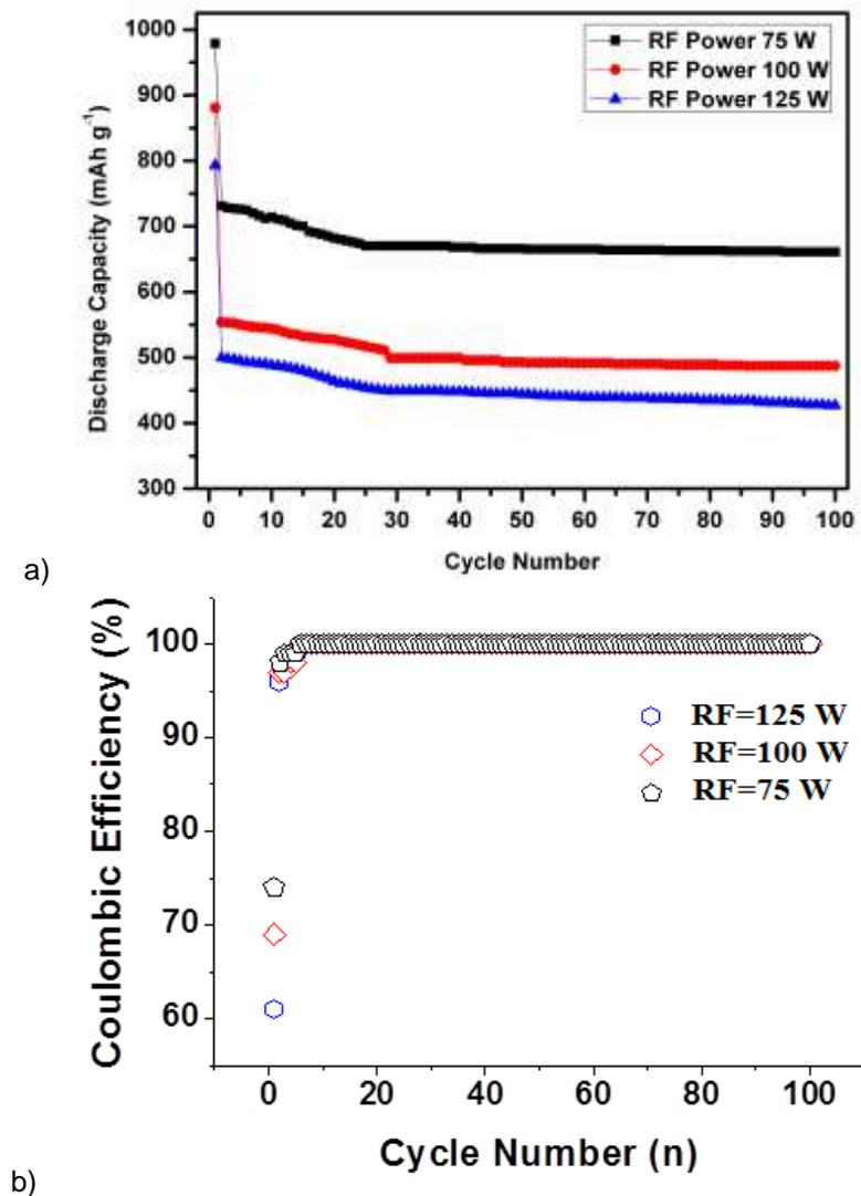
Figure 8. a) Discharge capacity – cycle diagram for the nanocomposite electrodes deposited under different plasma powers and b) Coulombic efficiencies of the electrodes.
