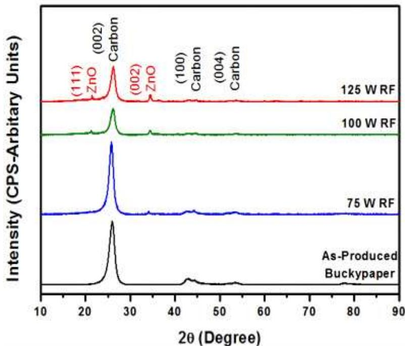
Figure 4. XRD patterns of bare buckypaper and ZnO/MWCNT nanocomposites deposited at various RF powers.
