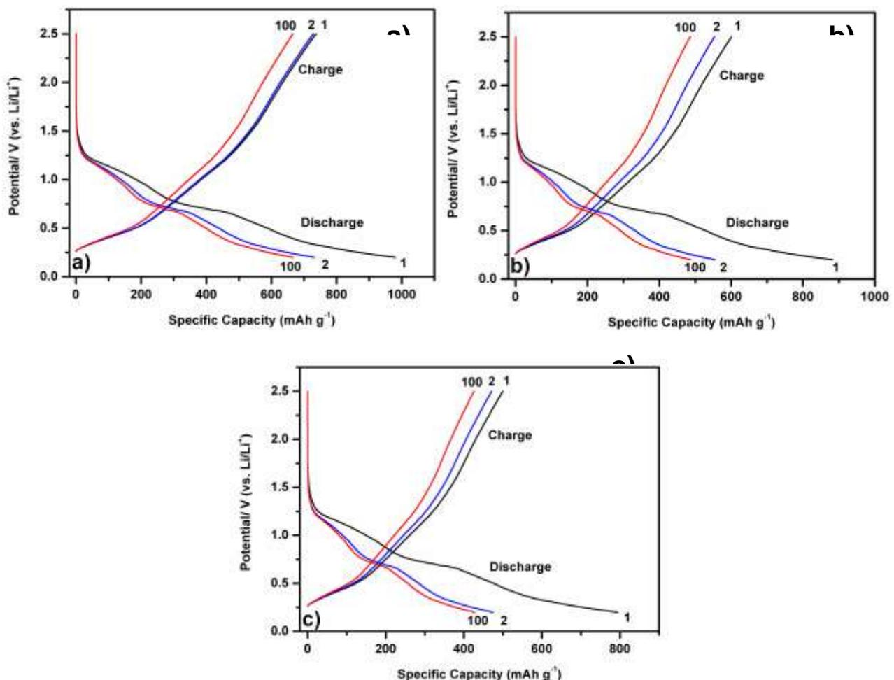
Figure 7. Galvanostatic charge-discharge curves of the films deposited at different RF powers; a) 75 W, b) 100 W and c) 125 W.
