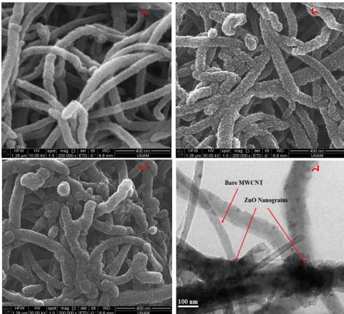
Figure 2. FESEM images of the films produced on the MWCNTs under different RF plasma powers; a) 75 W, b) 100 W, c) 125 W and d) TEM images of ZnO/MWCNT nanocomposite structure showing core-shell structure.
