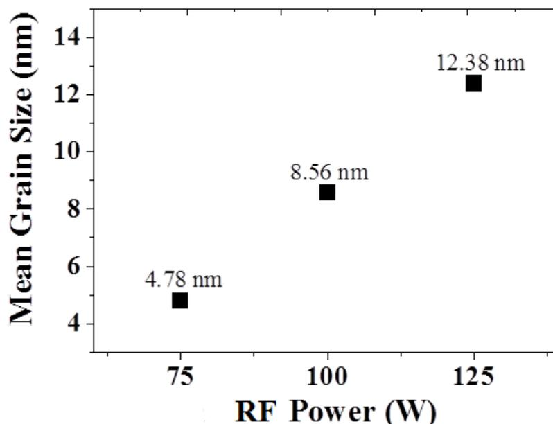
Figure 6. Mean grain sizes of the ZnO films deposited at various RF plasma powers.
