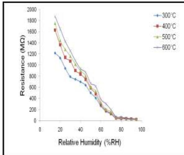
**Fig.5** Variation of resistance with change in % RH for the sensing elements AZ-8 annealed at different temperatures for humidification process.
