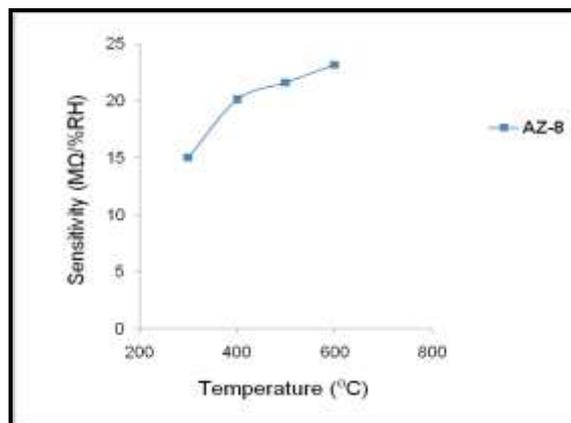
**Fig.6** Variation of Sensitivity with Temperature for the sensing elements AZ-8 annealed at different temperatures for humidification processes.
