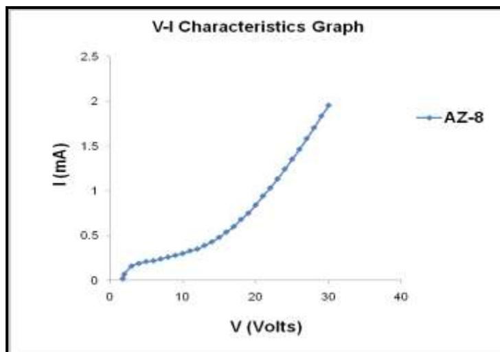
**Fig.2** V-I Characteristics Graph for sample AZ-8.
