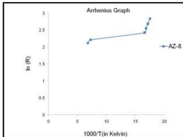
**Fig.1** Arrhenius Graph for Activation Energy for sample AZ-8.
