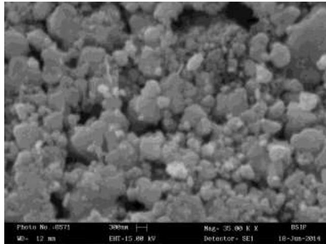
**Fig.3** SEM of sample AZ-8 annealed at 600°C.
