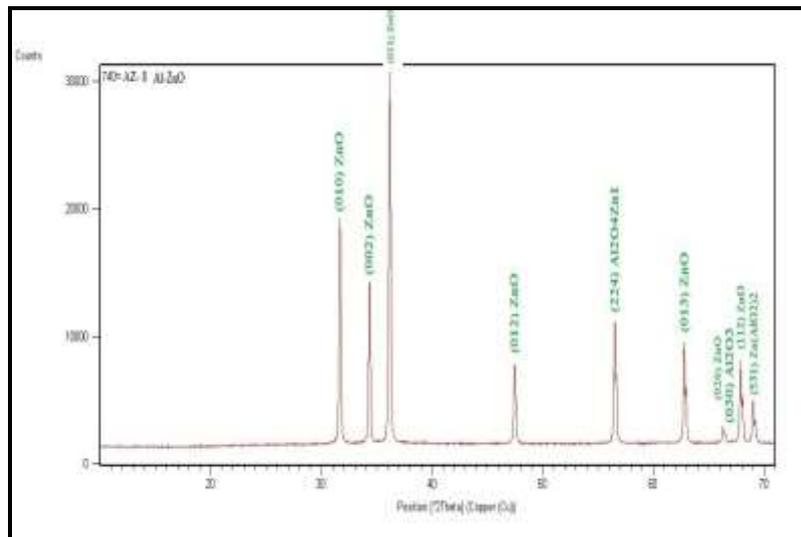
**Fig.4** XRD of sample AZ-8 annealed at 600°C.
