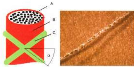
**Fig. 2** Schematic diagram of a composite yarn, A: base yarn, B: nanofiber layer, C: protective yarn [11]
