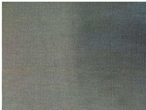
**Fig. 3** Woven fabric with nanofiber-covered yarn
