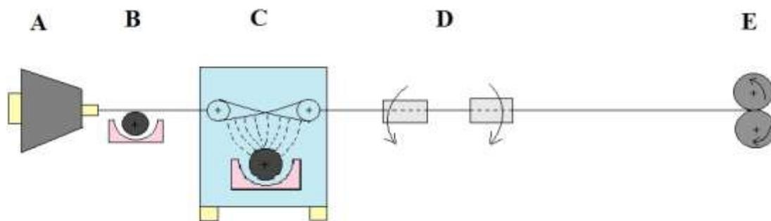
**Fig. 1.** Schematic diagram of a continuous production device A: base yarn, B: application of a conductive solution, C: nano spider, D: application of protective yarn(s), E: take-up mechanism.
