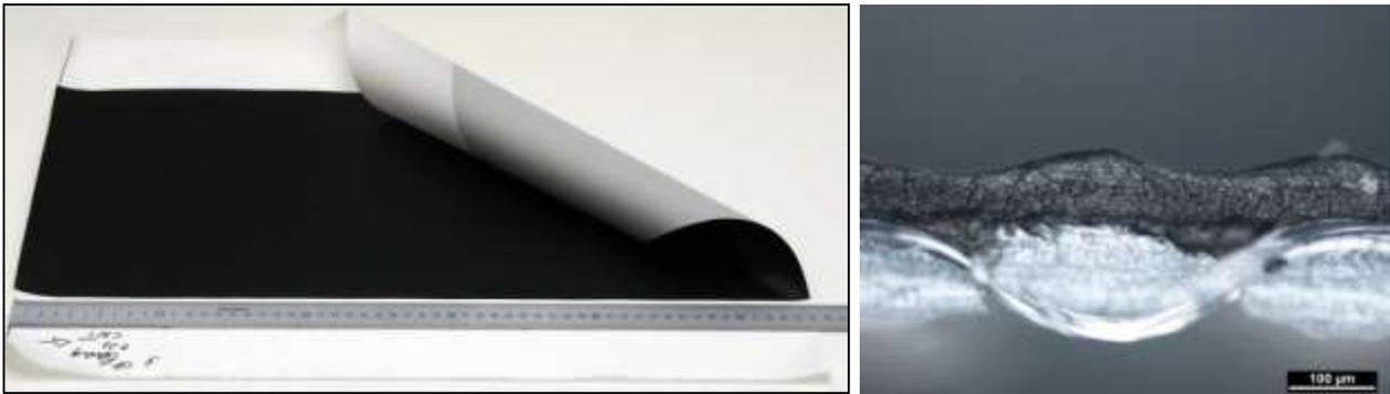
**Fig. 1** Black acrylate-based coating containing 10 wt% CNT on a white polyester fabric: as produced (left) and microscopic image of a cross section (right)
