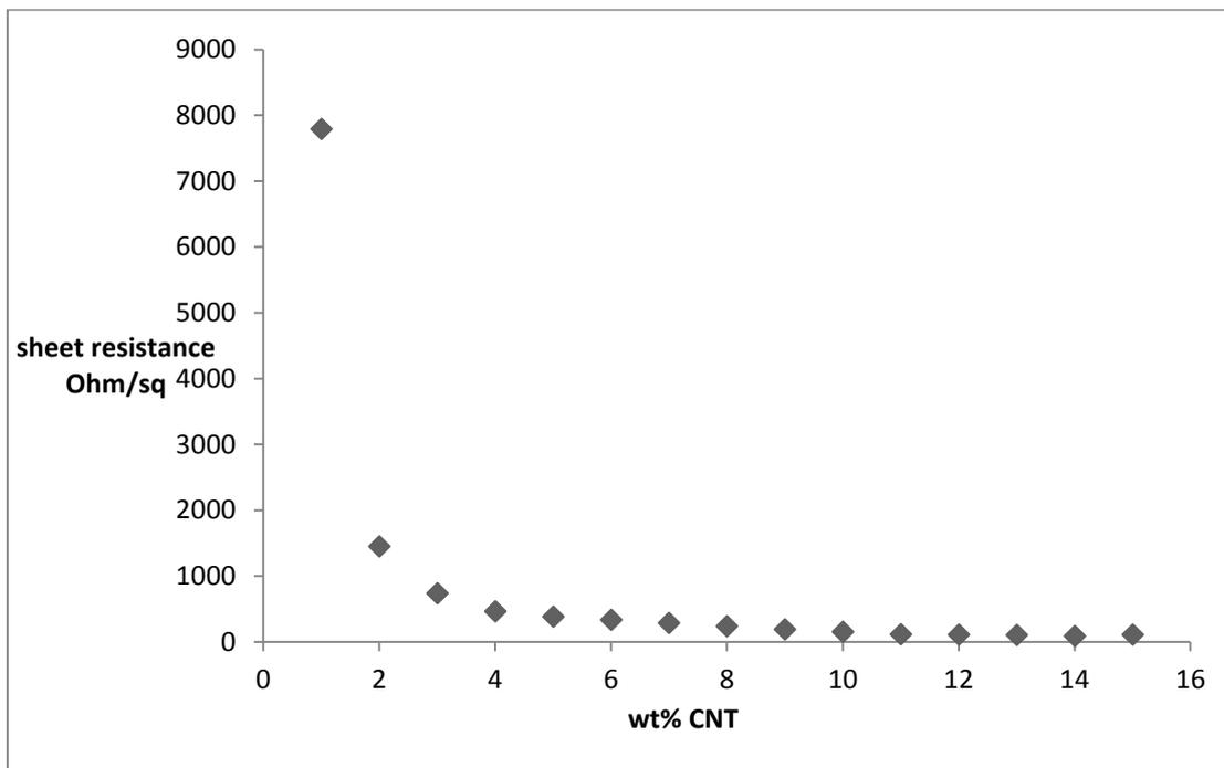
**Fig. 2** Sheet resistance of an acrylic-based textile coatings with different CNT loading (wt%)
