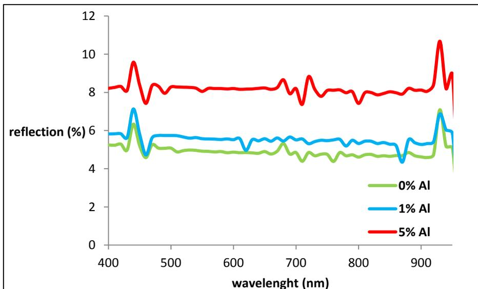
**Fig. 4** Reflection spectra of 10 wt% CNT based coatings with and without aluminium (Al)
