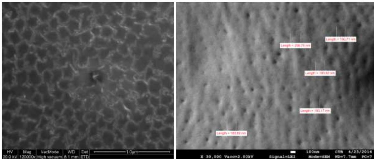
**Fig. 3** Scanning electron microscopy images of the surface of an acrylate-based coating containing 10 wt% CNT (left) and without CNT (right)
