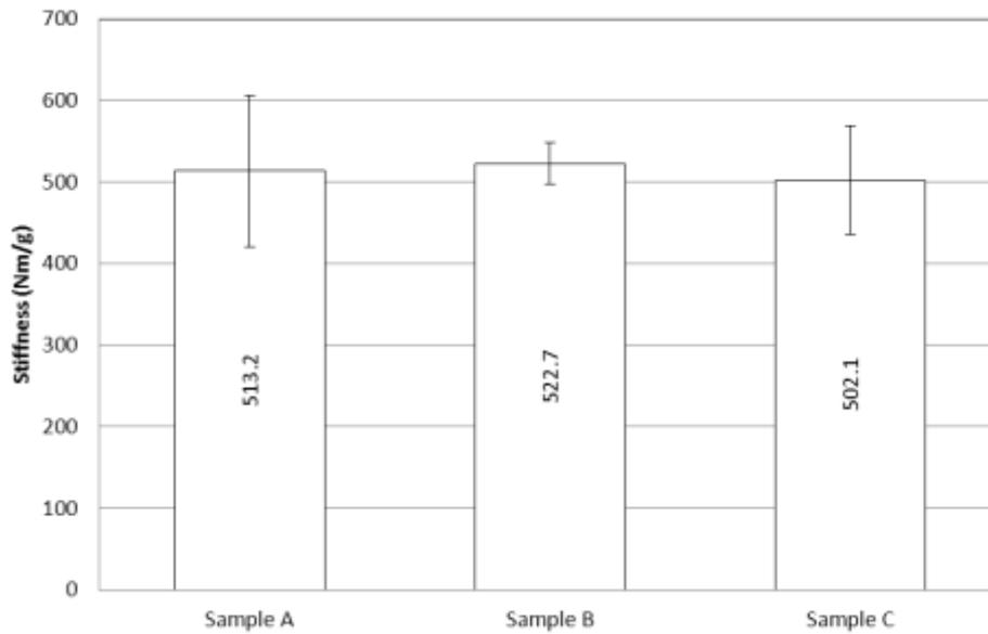
**Fig. 2:** Comparison of stiffness parameters for the tested nanofiber textiles.
