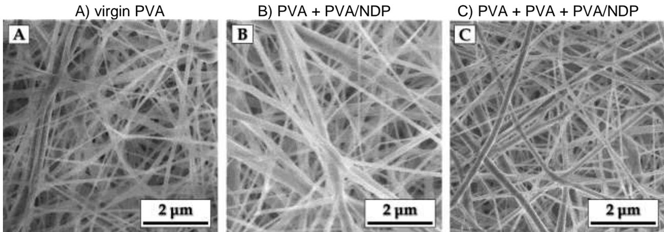
**Fig. 1:** SEM images of the tested nanofiber textiles (from left to right): samples A, samples B and samples C. All samples were thermally stabilized, scale bar is 2 µm.
