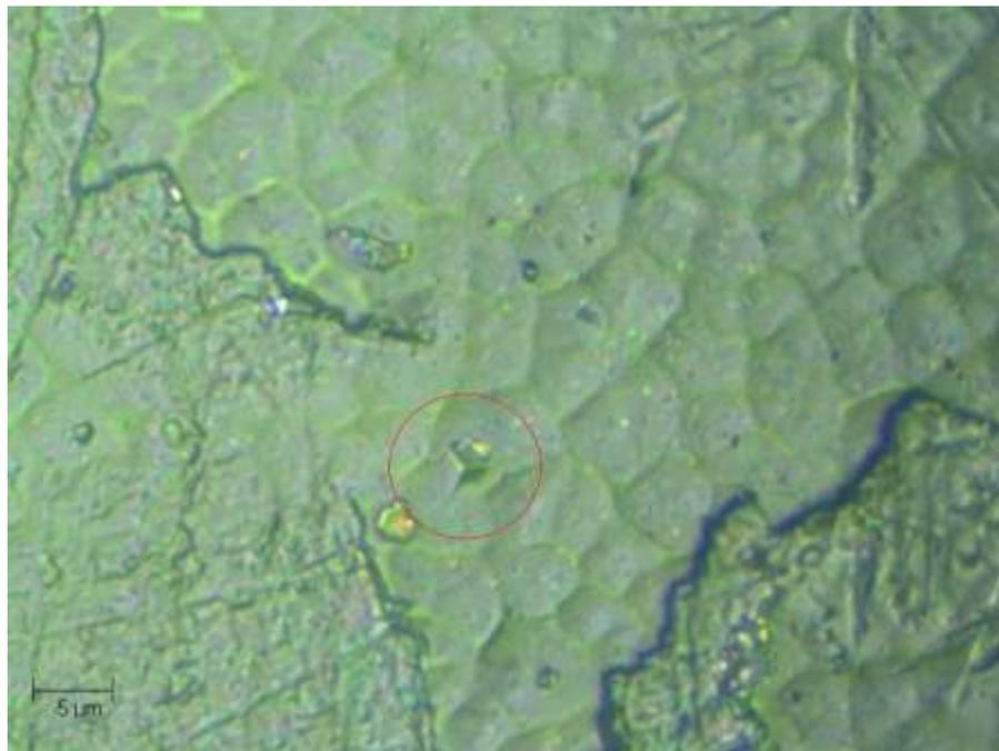
**Fig. 5** A visible puncture by a nano hardness tester into the sample evaluated, with the puncture location clearly shown. The sample size is 63  $\mu\text{m}$   $\times$  47  $\mu\text{m}$ .
