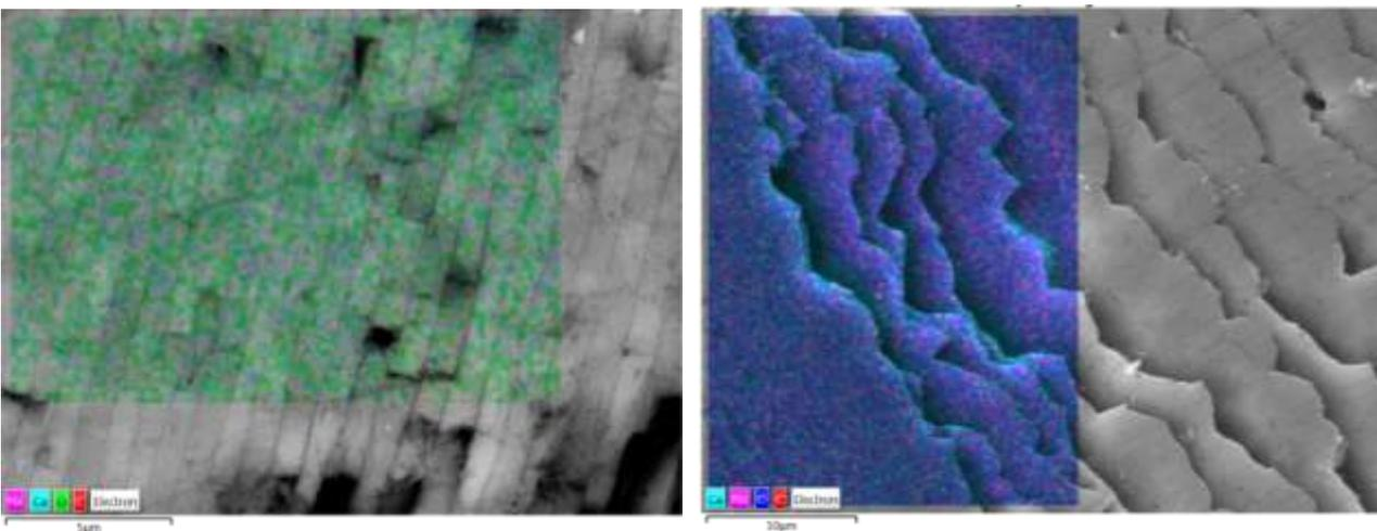
**Fig. 4** EDX analysis – Vertical and horizontal arrangement of plates in layers.
