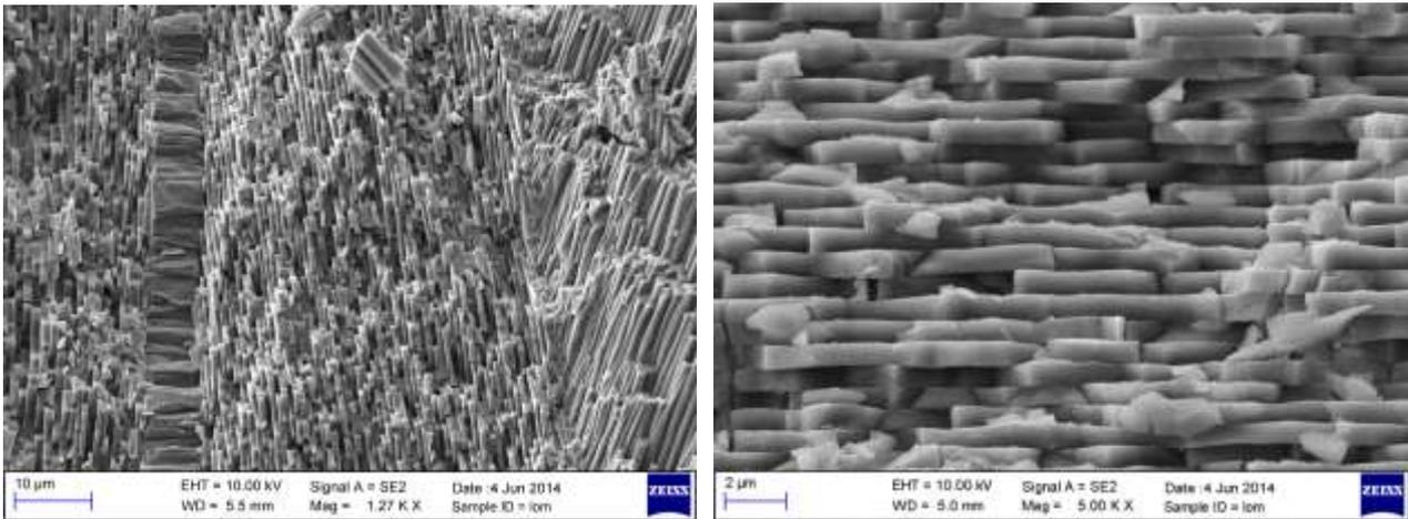
**Fig. 2** Plate arrangement – Fracture area and a fracture area detail.
