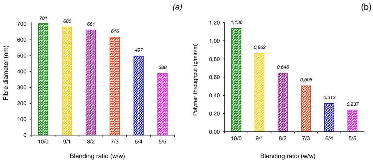
**Fig. 3** Effects of blend ratio of SF/PCL on (a) average fibre diameter; (b) spinning performance.
