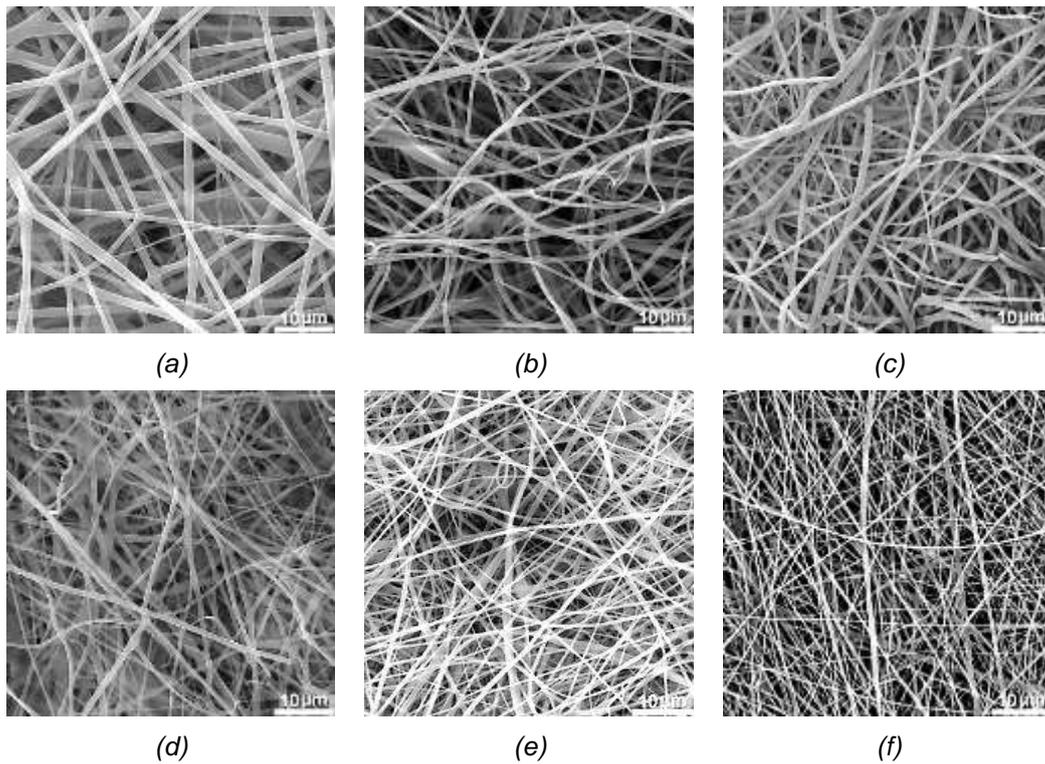
**Fig.2** SEM micrographs of SF/PCL blend fibres prepared from SF/PCL solution at various weight ratios. a) 10/0; b) 9/1; c) 8/2; d) 7/3; e) 6/4; f) 5/5
