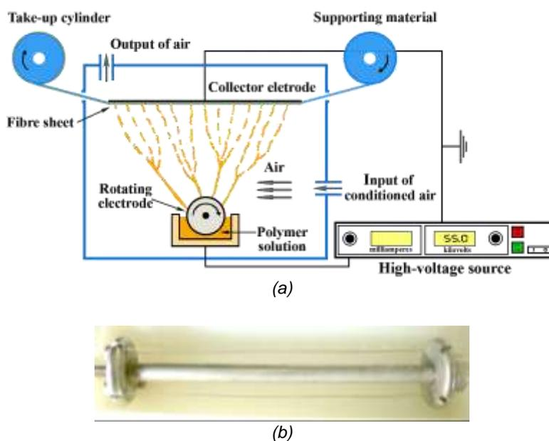
Fig. 1 (a) Schematics of needlesh electrospinning system, (b) a spinning electrode.
