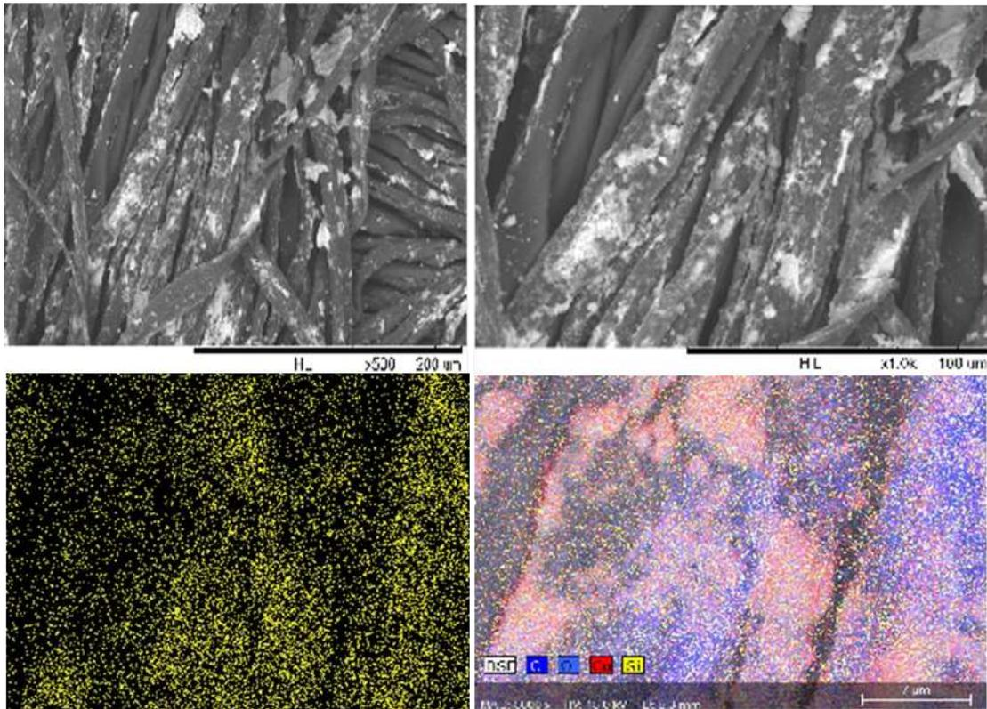
**Fig. 1** SEM micrographs of CuO nanoparticles on woven cotton fabrics
