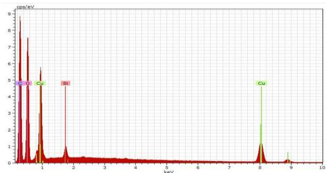
**Fig. 2** EDAX spectrum of CuO nanoparticles on woven cotton fabric
