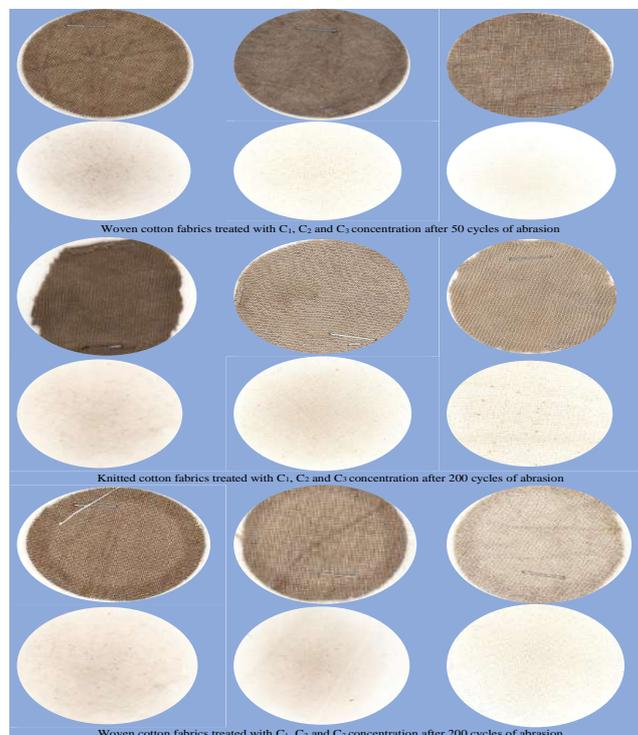
**Fig. 3** Abrasion resistance of treated fabrics
