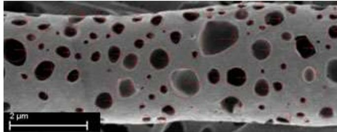
**Fig. 2.** HR SEM image of electrostatically spun fiber of 16% PCL.
