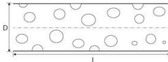
**Fig. 3.** A schema of porous fibre, where  $l$  is measured length and  $D$  is its diameter.
