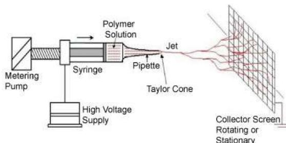
Fig. 1. Schematic diagram of electrospinning apparatus.
