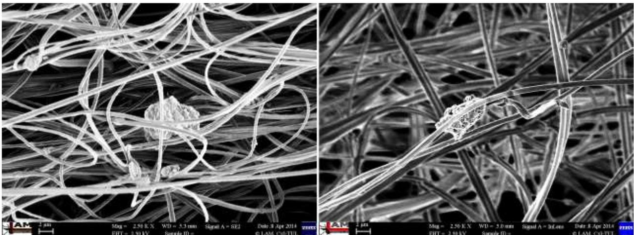
**Fig. 1** Cerium (left) and praseodymium (right) tungstates within PVB nanofibers, topographical contrast
