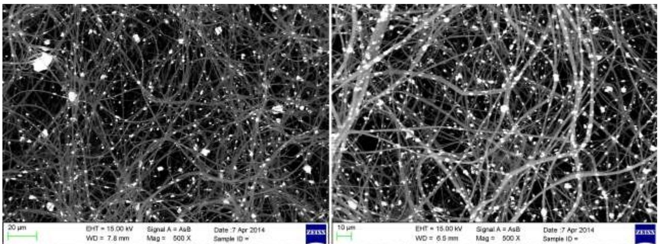
**Fig. 2** Cerium (left) and praseodymium (right) tungstates within PVB nanofibers, chemical contrast
