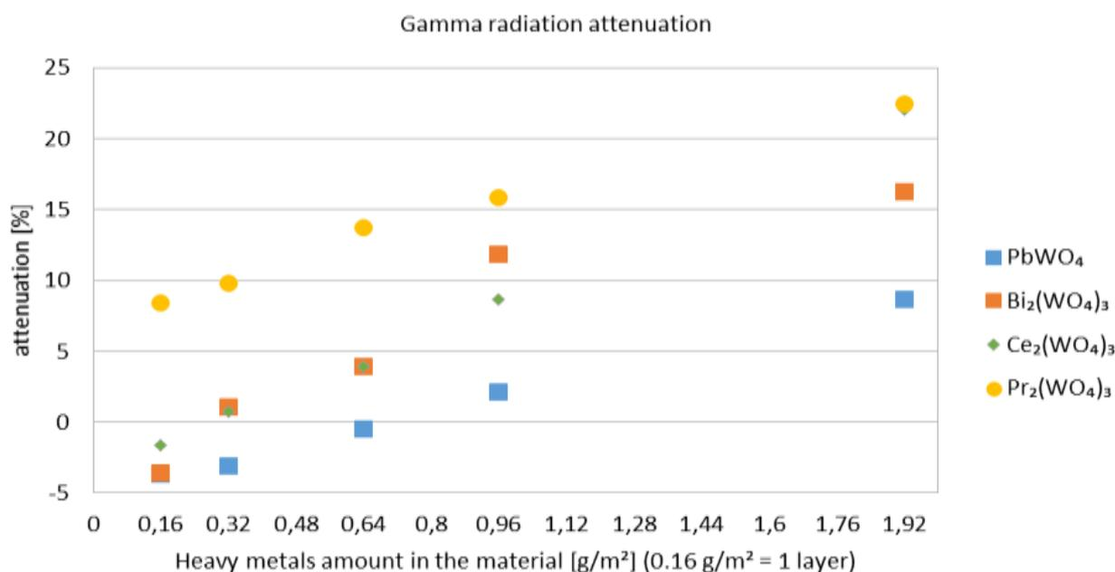
**Fig. 5** Gamma radiation attenuation while passing through the layers of composite material
