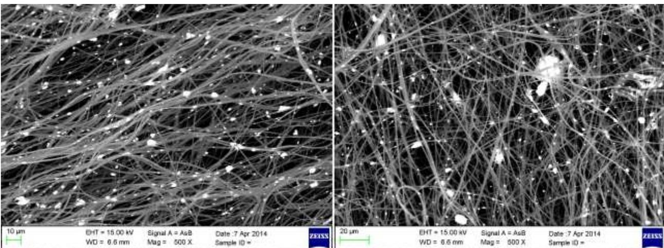
**Fig. 4** Lead (left) and bismuth (right) tungstates within PVB nanofibers, chemical contrast
