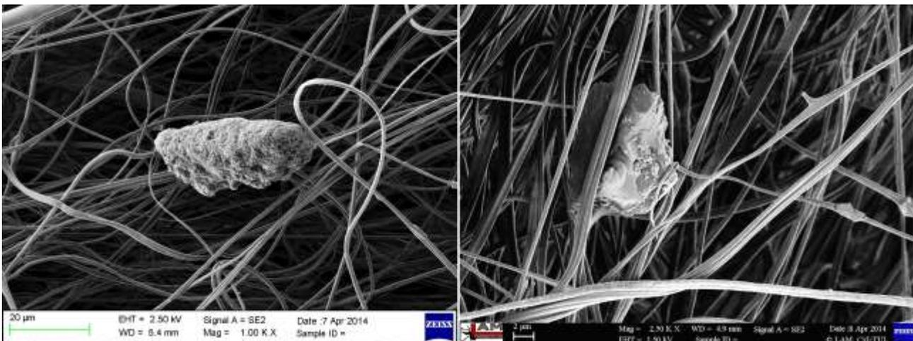
**Fig. 3** Lead (left) and bismuth (right) tungstates within PVB nanofibers, topographical contrast
