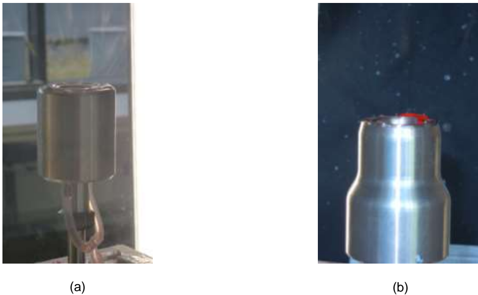
Fig. 3 Modification of the cylindrical coaxial spinning electrode (a) previous construction, (b) new construction.
