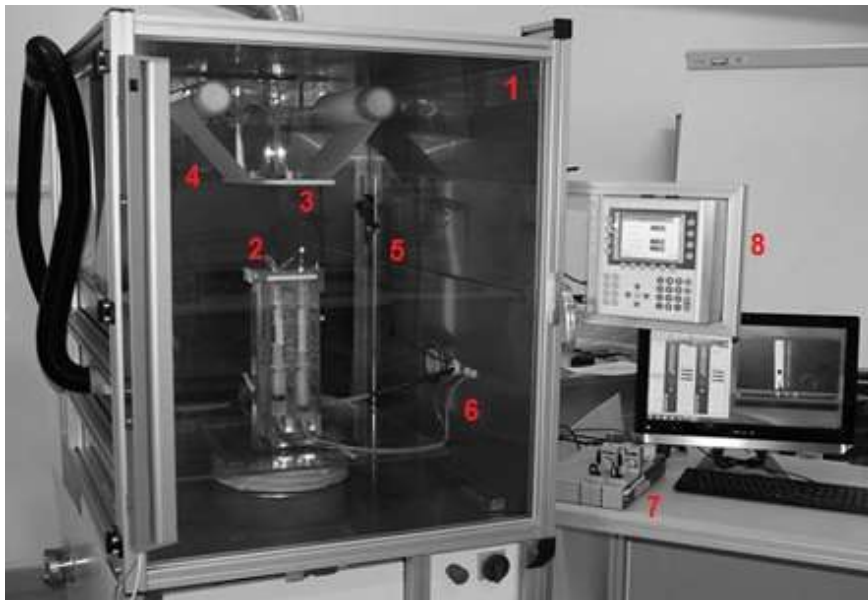
Fig. 1 Electrospinning device which is suitable for commercial use: (1) coaxial electrospinning device, (2) spinning electrode, (3) the collector, (4) the substrate material, (5) webcam for process control, (6) dosing system, (7) dosing pump, (8) the control panel.
