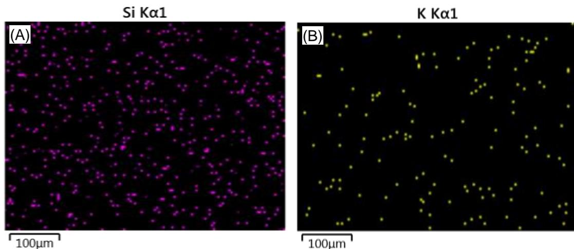
**Fig. 4** EDX analysis of a ChS Epoxy 520 epoxy resin system – filler at 0.5 phr performed for: **(A)** silicon, **(B)** potassium
