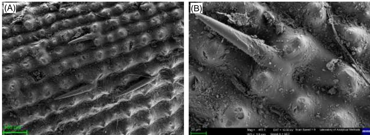
**Fig. 1** SEM image of the rice husk surface: (A) low magnification, (B) high magnification
