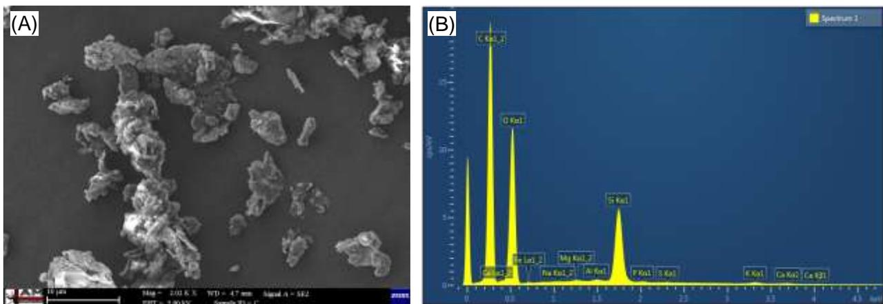
**Fig. 3** Ground material characteristics: **(A)** SEM of filler particles – rice husks, **(B)** EDX analysis of filler particles obtained by grinding from input material
