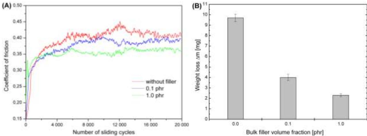
**Fig. 5** Tribological behaviour of epoxy resin composite systems: **(A)** Relationship between the coefficient of friction and filler volume; **(B)** Influence of the filler volume on the reduced wear rate in a hardened specimen from epoxy resin
