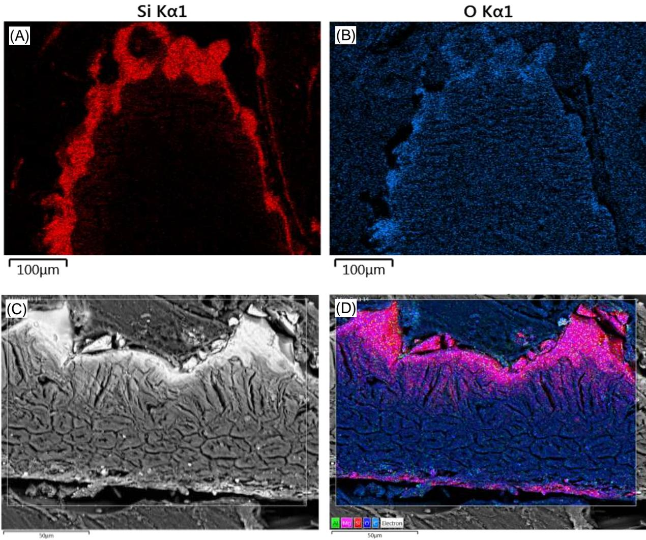
**Fig. 2** EDX analysis showing the distribution of elements typically found on the surface of rice husks: **(A)** silicon, **(B)** oxygen, **(C), (D)** silicon dioxide in superficial projections
