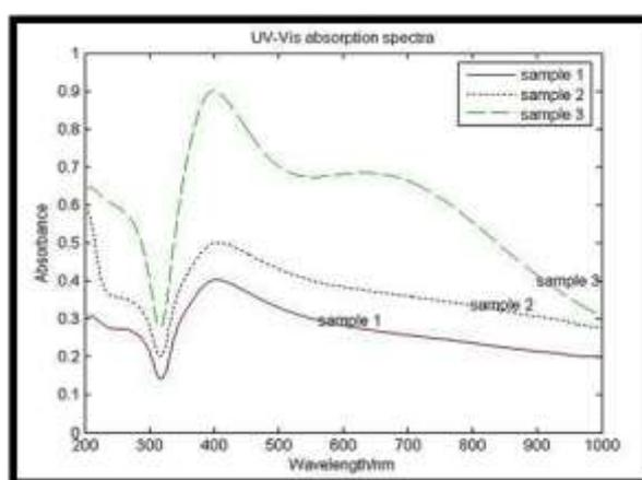
**Fig.3** UV-Vis absorption spectra of Ag- NPs in distilled water.
