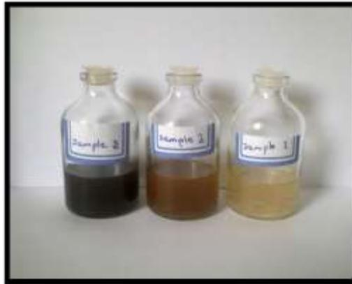
**Fig.1** Ag nanoparticles samples in distilled water.
