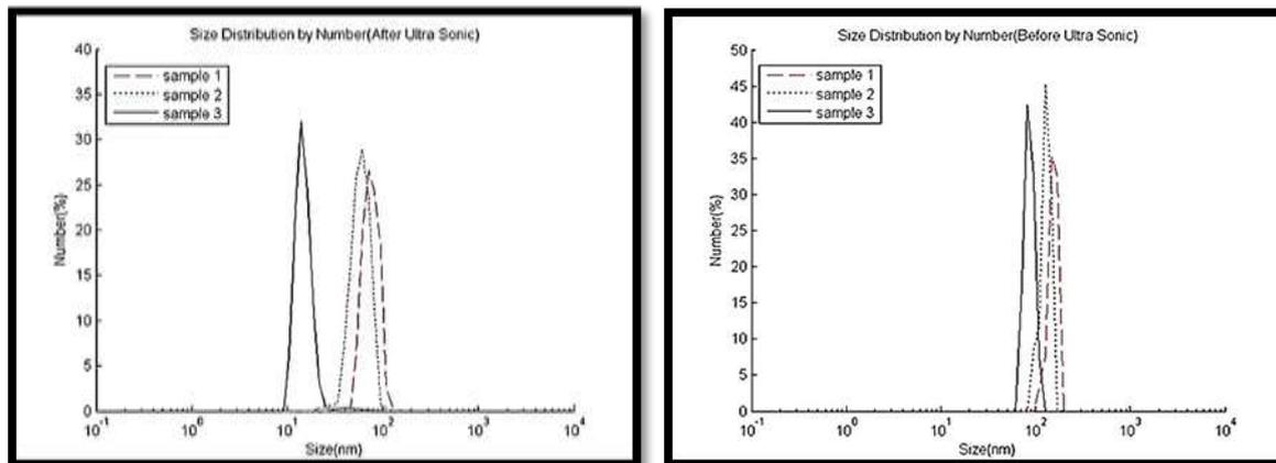
**Fig.5** Ag-NPs, hydrodynamic size distribution of samples measured by (DLS) before and ultrasonic treatments.
