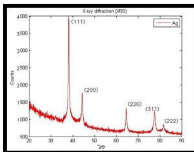
**Fig.2** X-ray diffraction pattern of Ag- NPs after drying
