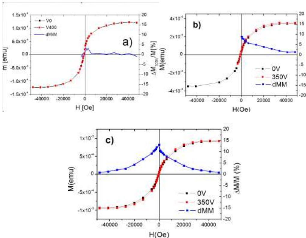
**Fig. 4** The changes of the in-plane hysteresis loop of a) 50 nm b) 130 nm c) 400 nm CSFO film grown on PMN-PT
