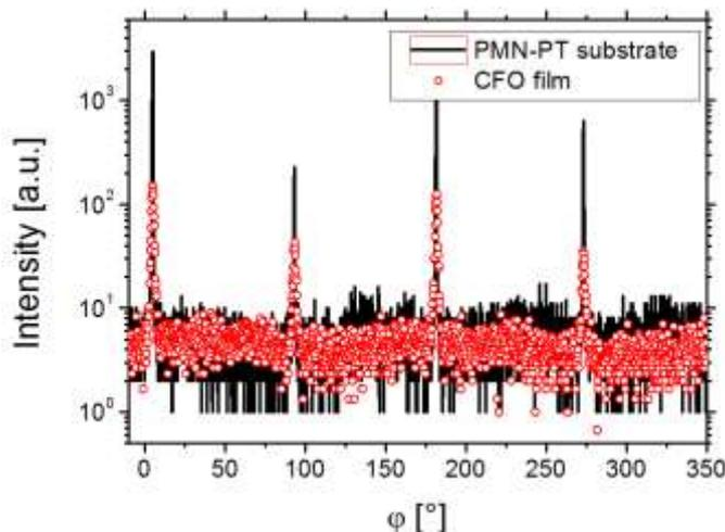
**Fig. 2**  $\phi$ -scans in (022) lattice plane of the cubic PMN-PT substrate and (044) of CSFO 400 nm film
