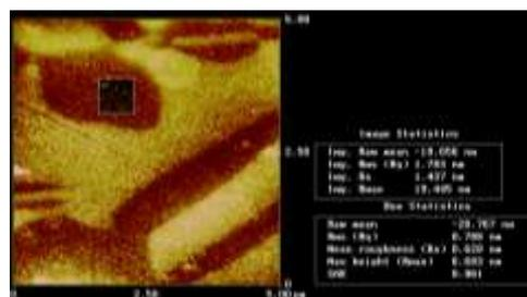
**Fig. 3** Surface morphology image of a 50 nm film taken by AFM
