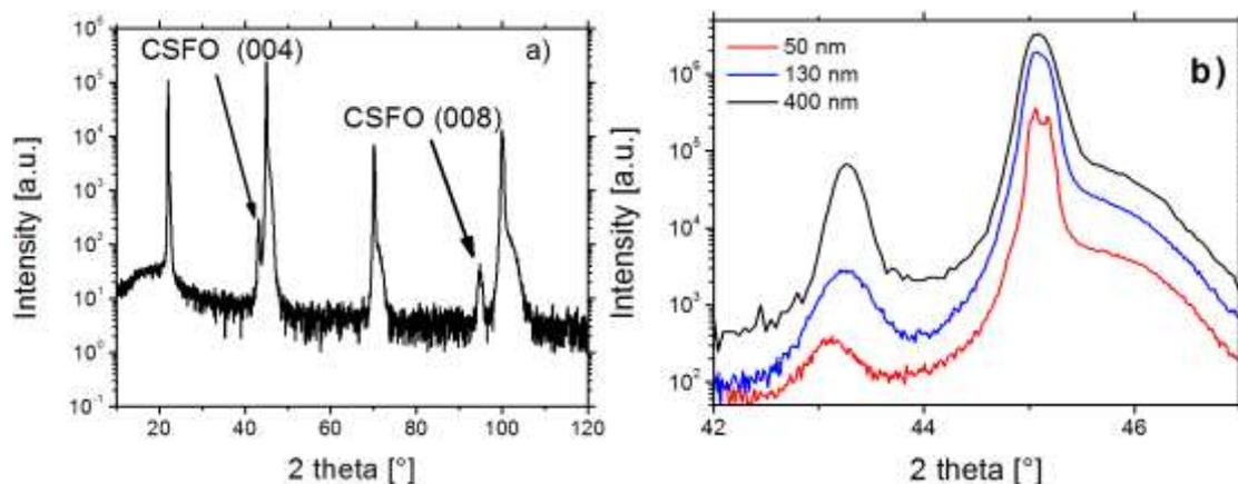
**Fig. 1 a)** X-ray diffraction patterns (Bragg-Brentano  $\theta$ - $2\theta$ ) of the 130 nm films on PMN-PT (001) and **b)**  $\theta$ - $2\theta$  scans around the substrate's (002) peak and CSFO film's (004) peak grown PMNPT
