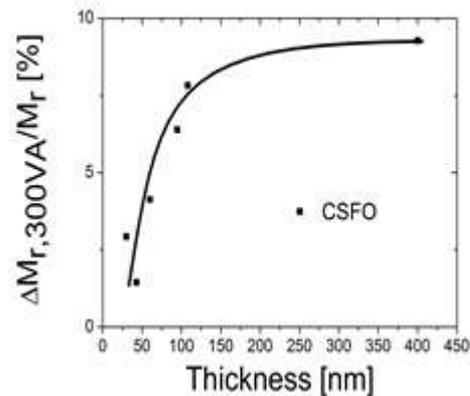
**Fig. 5** Strain-induced change of the in-plane remanent magnetization versus the thickness of the films
