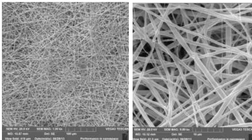
**Figure 2:** SEM scan of nano-fibrous textile before the test
