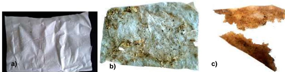
**Figure 3:** Biodegradation process of PHA-based nano-fibrous textile a) 0<sup>th</sup> hour b) 5 days c) 8 days
