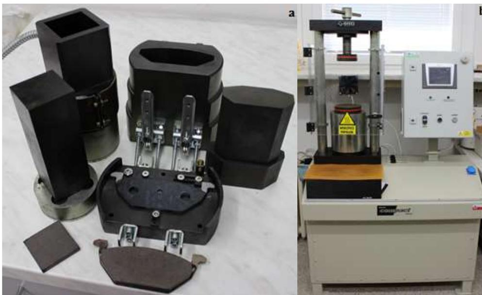
**Fig. 1** Brake pad pressing matrix (1a) and Compact Thermo 300 kN hot press (1b)
