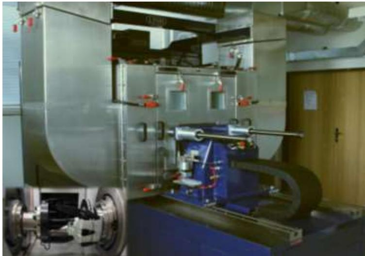
**Fig. 2** LINK M2800 compact full-scale brake dynamometer
