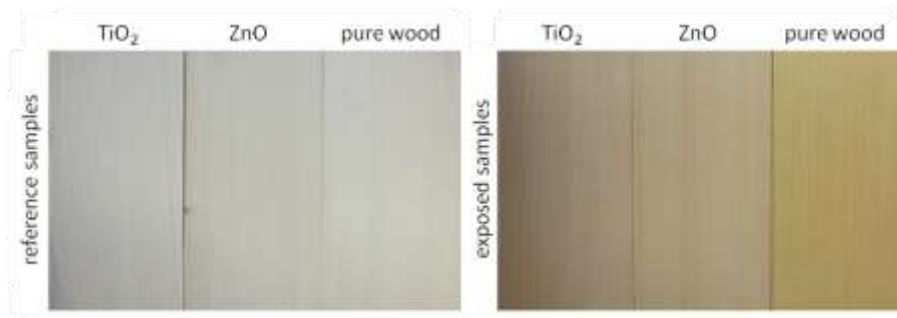
Fig. 4 Photos of wood (spruce) with or without protection coating before (on the left side) and after 4 month UV-C exposition (on the right side)
