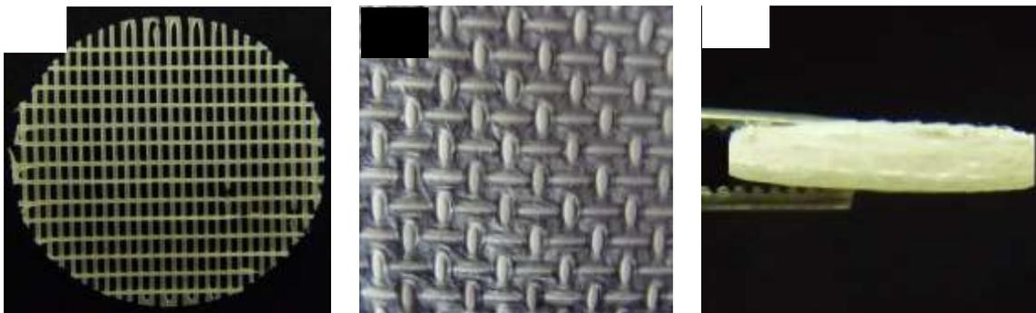
**Fig. 4** A photo of the special 3D printed layer (a), special patterned nanofibrous layer (b) and final scaffold – diameter 16mm, thickness 4mm (c)
