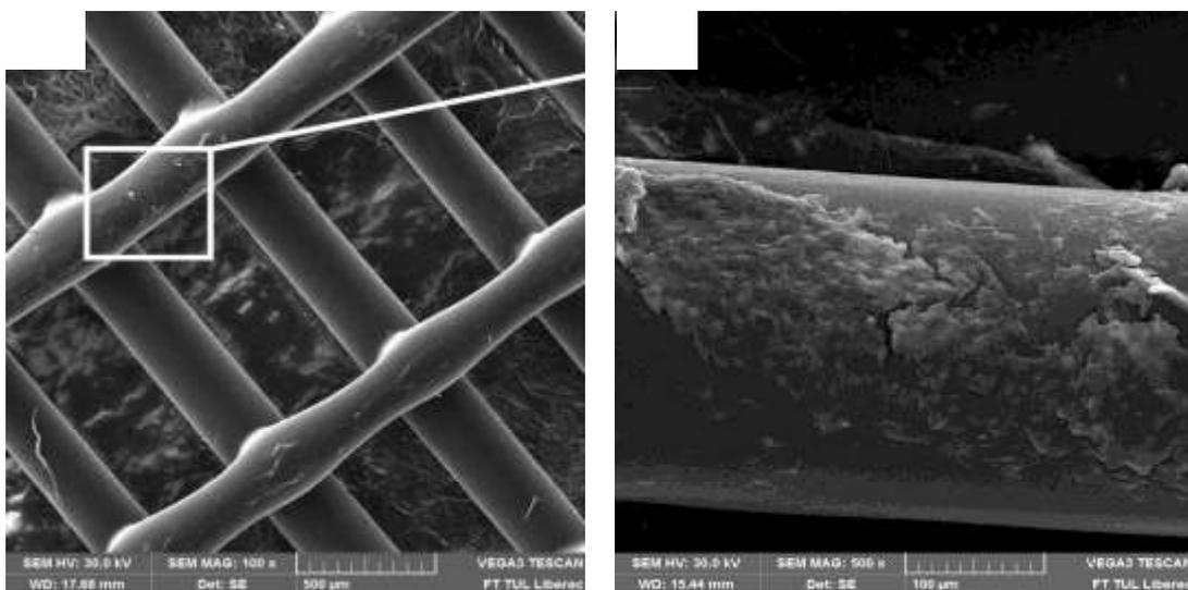
**Fig. 5** SEM image at day 14 – top view onto complete scaffold (a) and detail the marked area (b)
