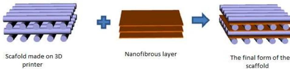
**Fig. 1** Schematic view of making a scaffold [2]
