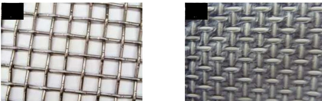
**Fig. 2** A photo of the special wire collector (a) used for production of patterned nanofibrous layer (b)
