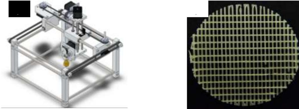
**Fig. 3** A photo of the special 3D printer (a) used for production of perpendicular laid structure
