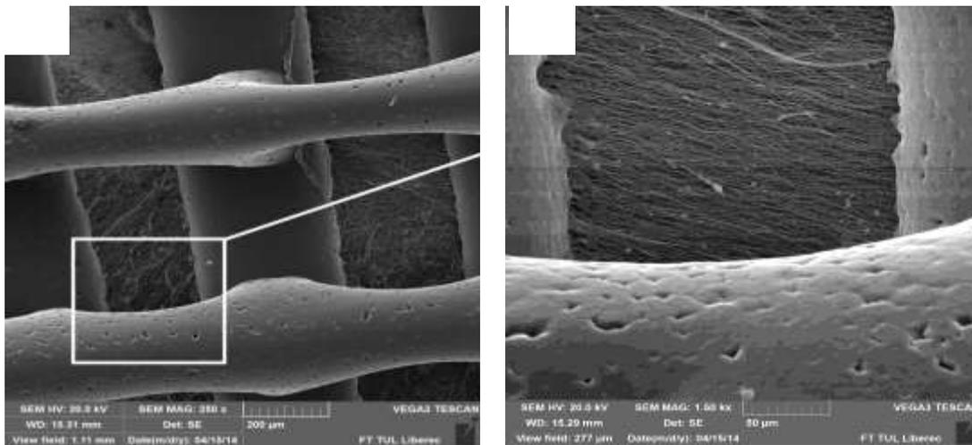
**Fig. 4** SEM image of top view onto scaffold combining 3D printing and patterned nanofibrous layers (a) and detail the marked area (b)
