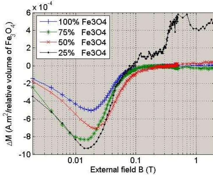
**Fig. 2** The Henkel plots. The influence of diamagnetic matrix composed from fine MgO powder on interparticle magnetic interactions in single domain magnetite (particle size smaller than 50 nm).
