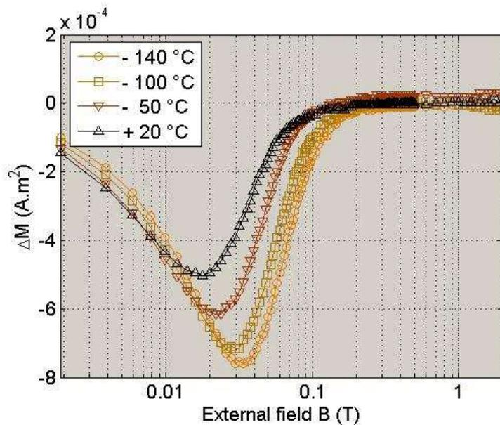
**Fig. 1** The Henkel plots. The influence of temperature on interparticle interactions in the powder that consists of particles of single domain magnetite (particle size is smaller than 50 nm).
