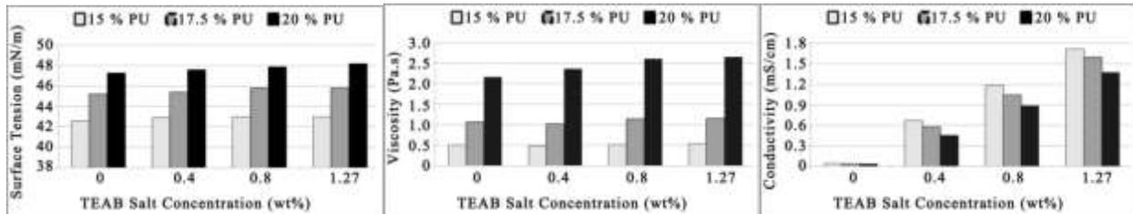
**Fig. 2** Surface tension, viscosity, conductivity of PU solutions
