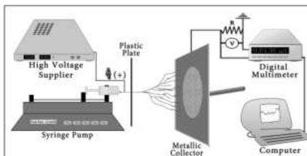
**Fig 1** Electrospinning setup
