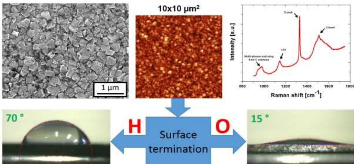
**Fig. 1** SEM image, AFM image and Raman spectrum of the diamond film (top row), and wetting properties of the H-terminated and O-terminated diamond surface (bottom row).
