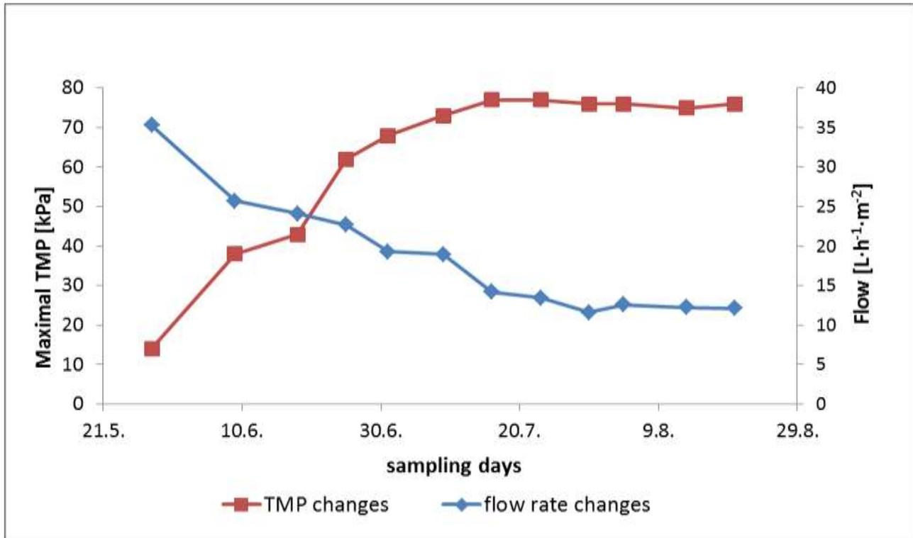
Fig. 4: Pressure and filtration velocity changes during Pilot run
